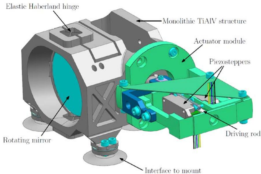
**Figure 2. CAD model of the latest IFPM design.**
