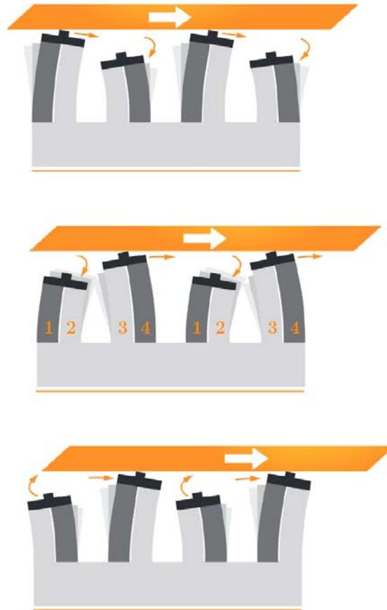
**Figure 1. Operating principle of the walking piezo actuator. Due to the ellipsoidal movement of the tip of the legs, the ceramic rod moves in horizontal direction. The numbers indicate the phases; same-phase piezos are fed with the same voltage. Image courtesy of PiezoMotor®.**
