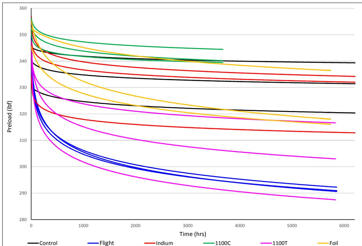
Figure 4. Curve Fits for Preload Loss Over Time
