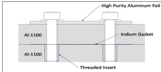
Figure 1. Representative Heat Strap Bolted Joint Interface
