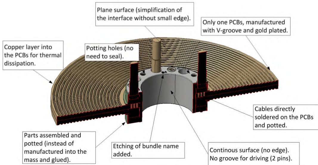
Figure 2. Rotor sub-assembly improvement
