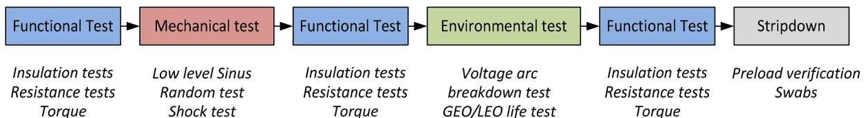
Figure 5. Qualification test sequence
