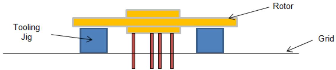
Figure 6. Rotor sketch assembly into the oven
