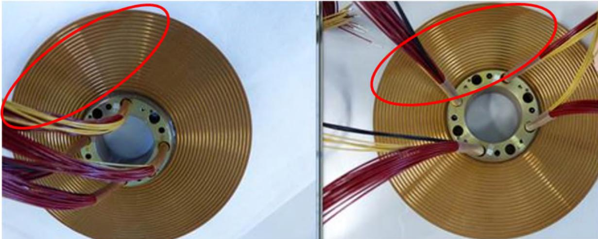
Figure 7. Discoloration on rotor track
