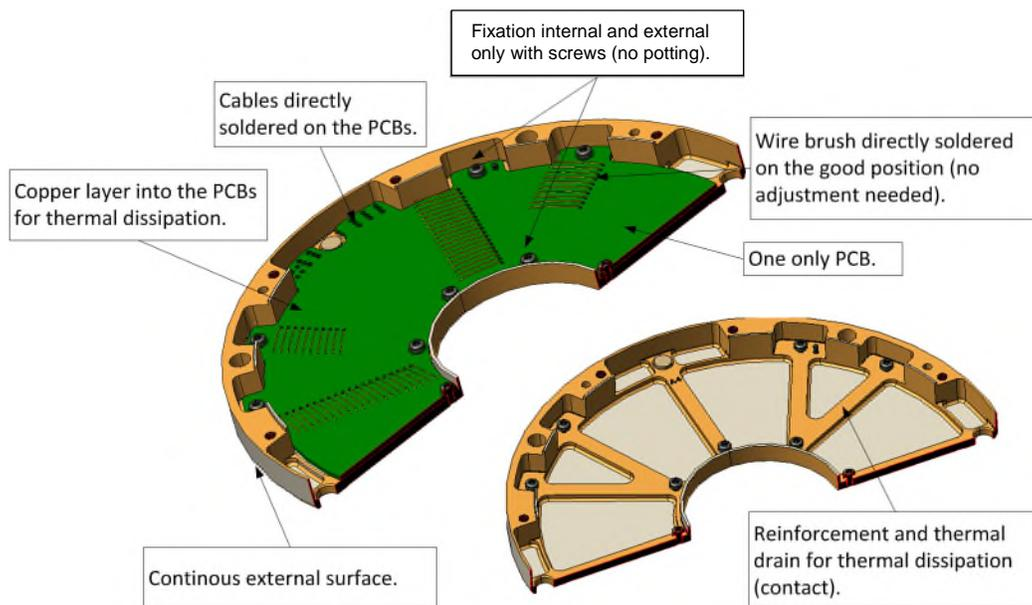
Figure 3. Stator sub-assembly improvement
