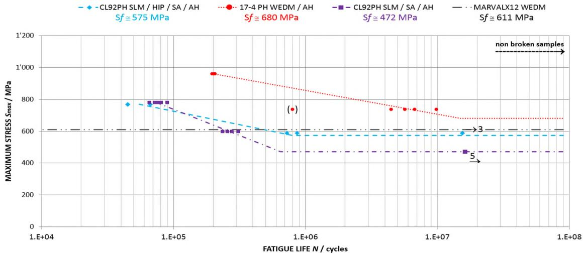
Figure 4. S-N curves estimates for SLM (CL92PH) and WEDM (17-4PH) samples. The fatigue limit of MARVALX12 was determined experimentally during the MTG-CCM test campaign.
