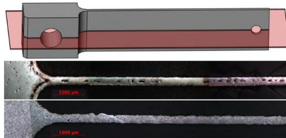
Figure 2. Fatigue sample cross-sections before and after SLM parameters optimization. The thickness of the blade is 350  $\mu\text{m}$ .
