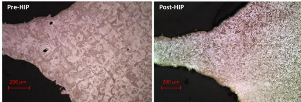
Figure 3. Sample cross-sections before and after HIP processing.
