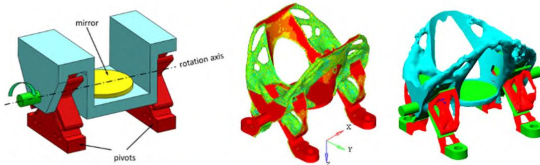
*Figure 8. Example of scanning compliant mechanism designed and optimized for monolithic additive manufacturing. Left: architecture overview, middle: first results without support material considerations, right: raw result with constrained parameters to avoid overhanging structure of less than 45° from horizontal plane.*
