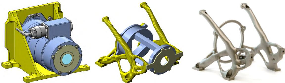
Figure 6. Example of CLUPI (EXO MARS Mission) bracket redesigned with topology optimization. Left: classical bracket, middle: geometry optimized to maximize the stiffness with a given mass diminution, right: part additively manufactured in titanium alloy.
