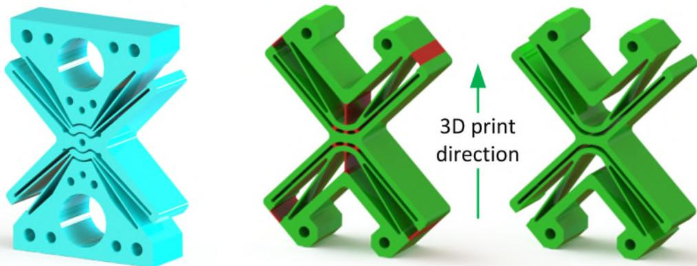
Figure 7. Example of HAFHA pivot redesigned for monolithic AM with a given print direction. Left: classical pivot, middle: optimized for AM with support bridges in red, right: AM pivot after bridge removal.
