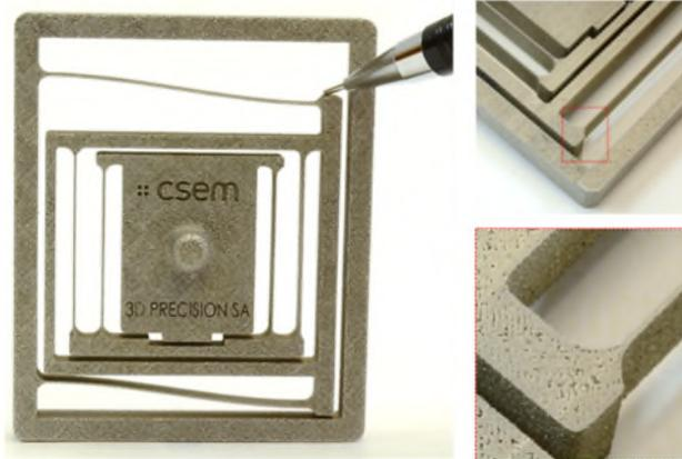
Figure 1. AM-SLM produced 316L stainless steel 2-DoF linear stage. Flexures thickness = 300  $\mu\text{m}$ , aspect ratio respectively 80 and 123 for the blades of the double and simple parallelograms
