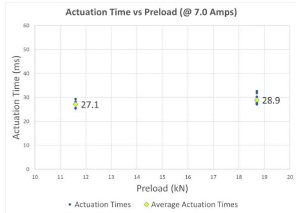
Figure 5. Actuation Time vs Preload
