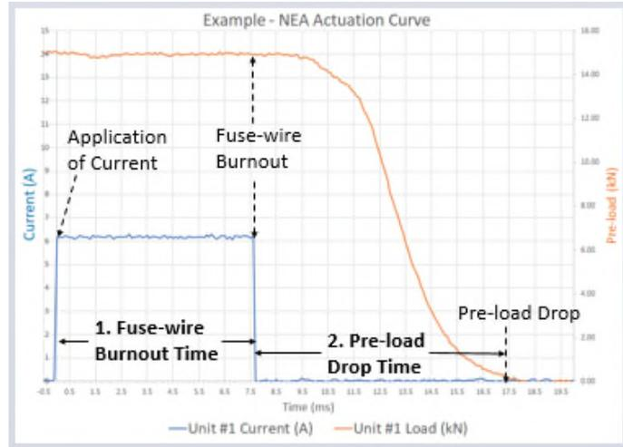
Figure 1. Example of Typical NEA Actuation Time Curve
