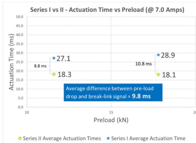
Figure 10. Series I (break-link) vs Series II (load cell) Actuation Time
