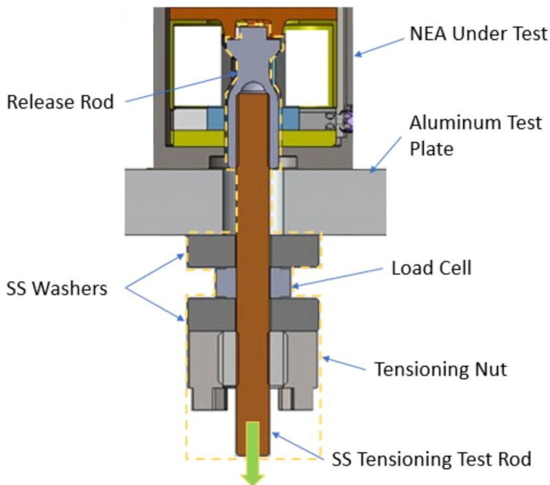
1. Tensioning Nut creates a tensile preload thru the test rod and into the NEA, compressing the Test Plate and Load Cell between the NEA and washers.
