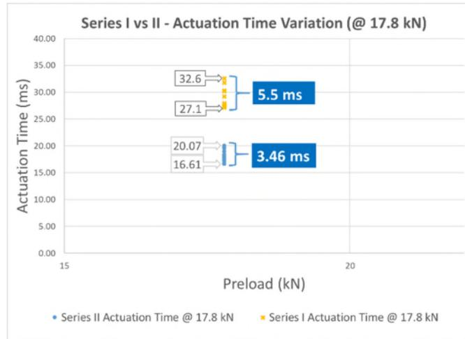
Figure 11. Series I (break-link) vs Series II (load cell) Actuation Time Variation
