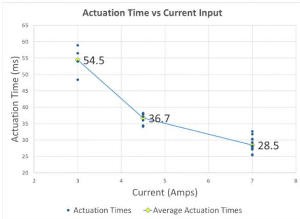
Figure 4. Actuation Time vs Current
