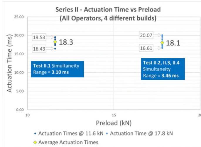
Figure 9. Series II Actuation Time vs Preload
