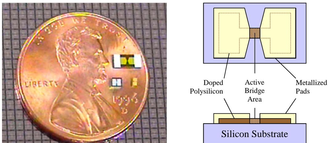
Figure 2. Semiconductor Bridge Construction
