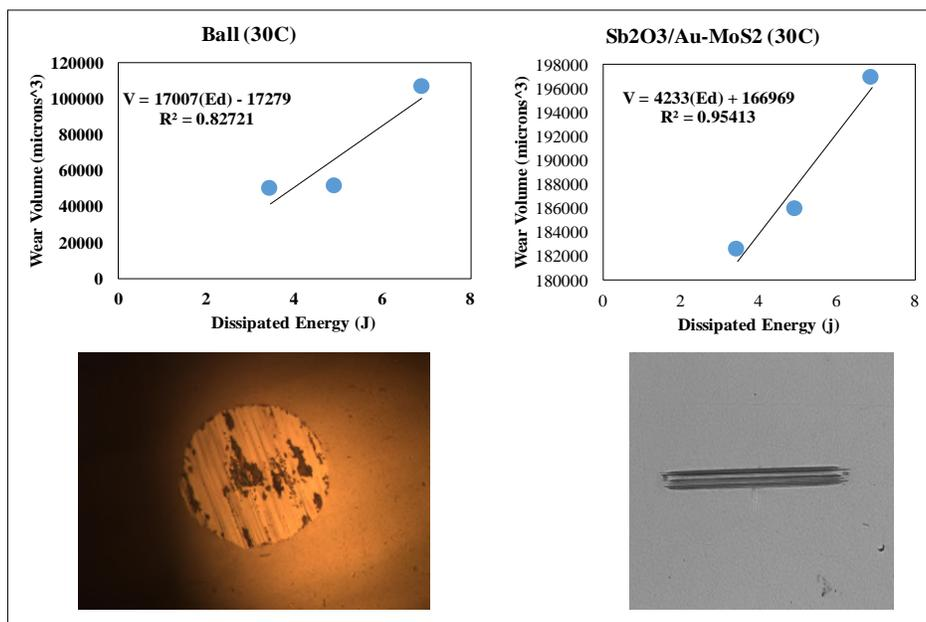
Figure 4, Wear volumes (*V*) for the Sb<sub>2</sub>O<sub>3</sub>/Au-MoS<sub>2</sub> coating and mated steel ball obtained from tests performed at 30°C are plotted against *E<sub>d</sub>* along with optical images of the wear scars on the ball and coating generated after 17,000 cycles. Lines in the figures are least square fits of Eq. 3 to the data.
