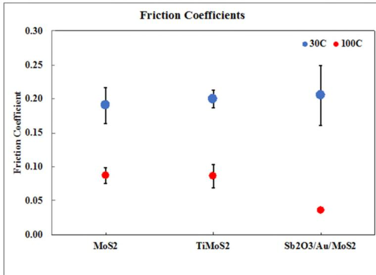
Figure 1. Average friction coefficients and standard deviations for the three coatings at 30°C and 100°C obtained in reciprocating sliding contact with a sliding amplitude of 1 mm, a frequency of 20 Hz, and a contact stress of 660 MPa.
