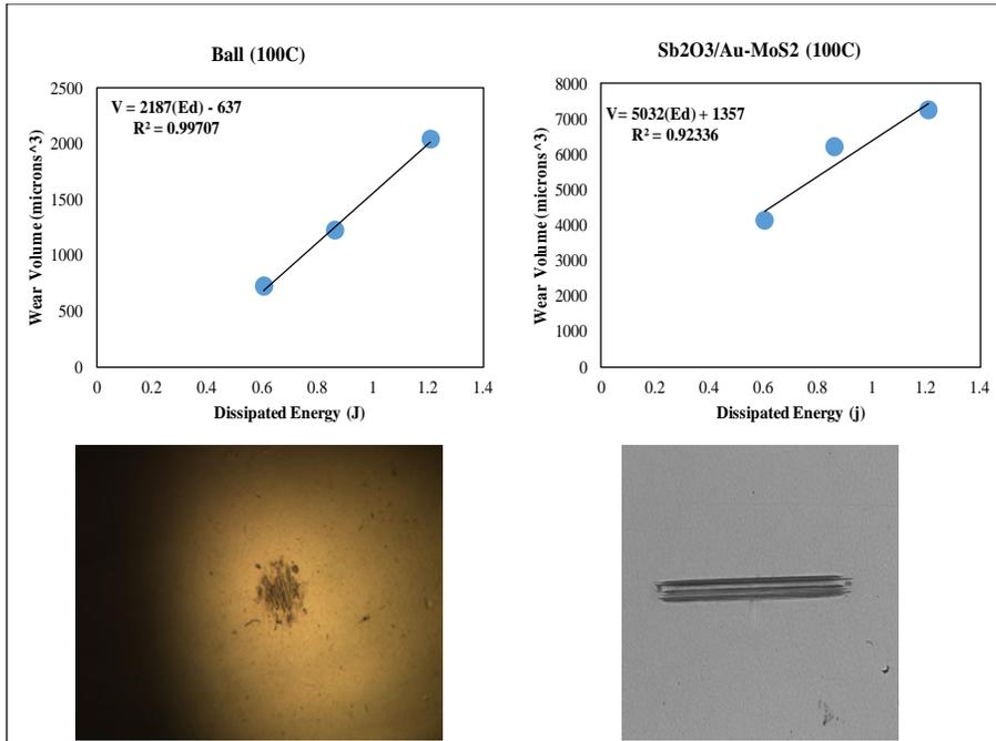
Figure 5, Wear volumes ( $V$ ) for the  $Sb_2O_3/Au-MoS_2$  coating and mated steel ball obtained from tests performed at 100°C are plotted against  $E_d$  along with optical images of the wear scars on the ball and coating generated after 17,000 cycles. Lines in the figures are least square fits of Eq. 3 to the data.
