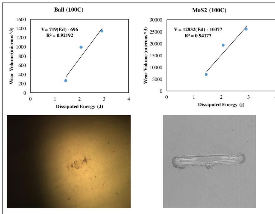
Figure 3. Wear volumes ( $V$ ) for the  $\text{MoS}_2$  coating and mated steel ball obtained from tests performed at  $100^\circ\text{C}$  are plotted against  $E_d$  along with optical images of the wear scars on the ball and coating generated after 17,000 cycles. Lines in the figures are least square fits of Eq. 3 to the data.
