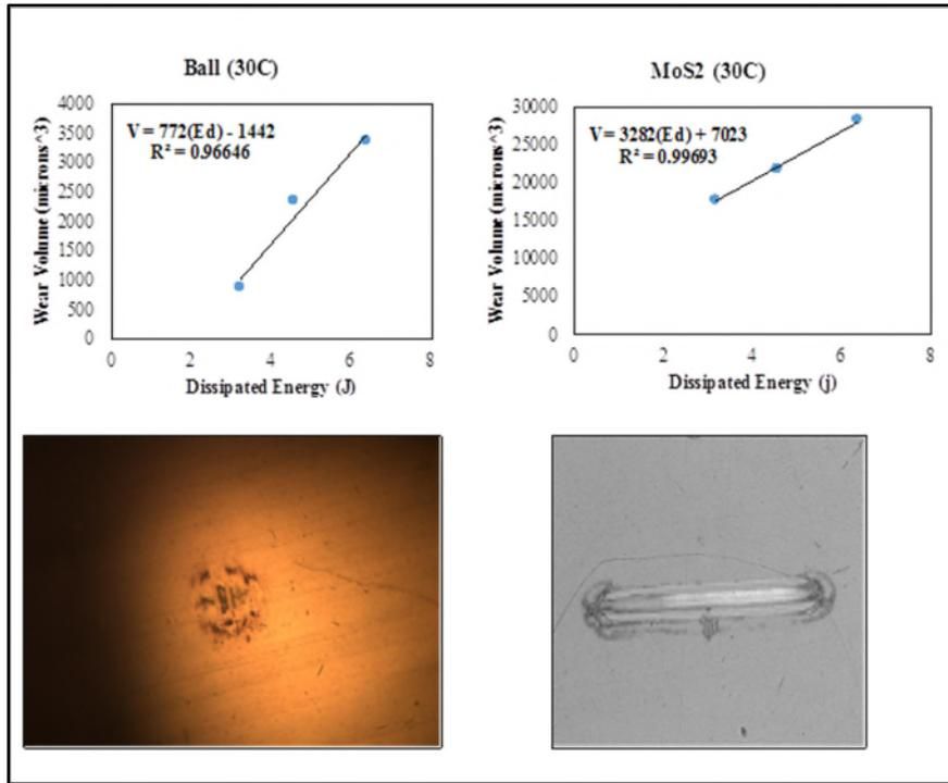
Figure 2. Wear volumes ( $V$ ) for the  $\text{MoS}_2$  coating and mated steel ball obtained from tests performed at  $30^\circ\text{C}$  are plotted against  $E_d$  along with optical images of the wear scars on the ball and coating generated after 17,000 cycles. Lines in the figures are least square fits of Eq. 3 to the data.
