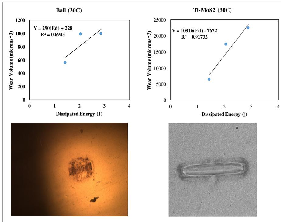
Figure 6, Wear volumes ( $V$ ) for the  $Ti-MoS_2$  coating and mated steel ball obtained from tests performed at 30°C are plotted against  $E_d$  along with optical images of the wear scars on the ball and coating generated after 17,000 cycles. Lines in the figures are least square fits of Eq. 3 to the data.
