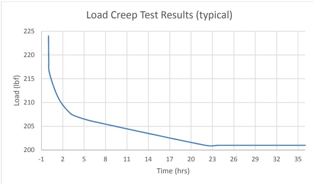
Figure 6. Load Creep Test Results
