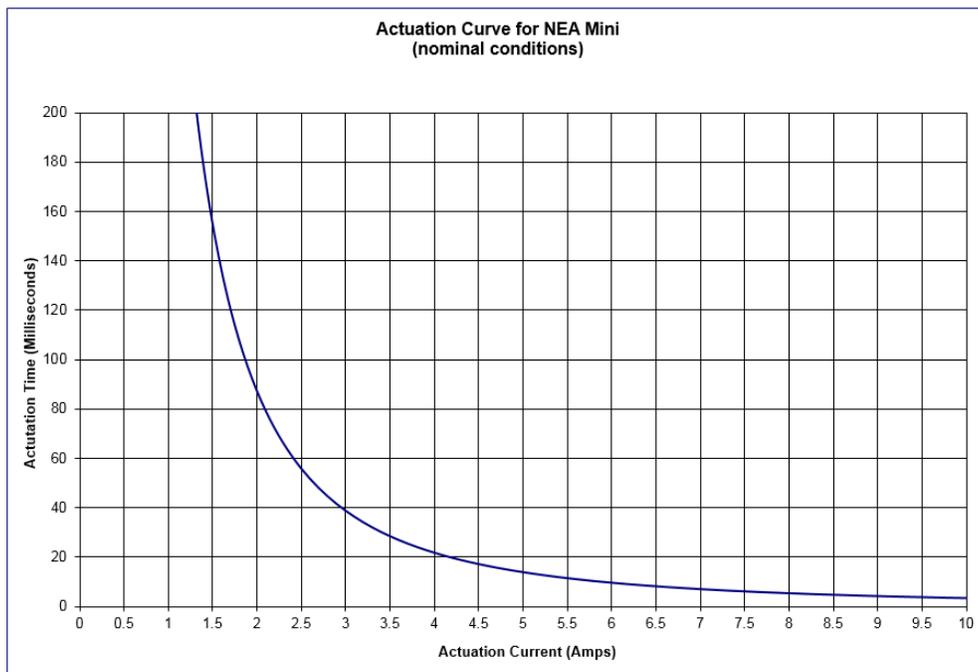
Figure 2. NEA Mechanism Actuation Curve
