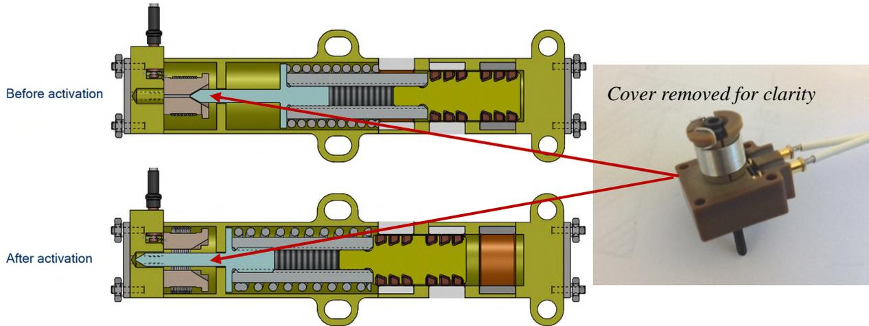
Figure 1. Battery bypass switch
