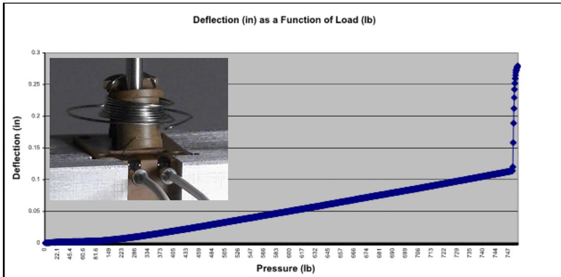
Figure 3. NEA Ultimate Load Test
