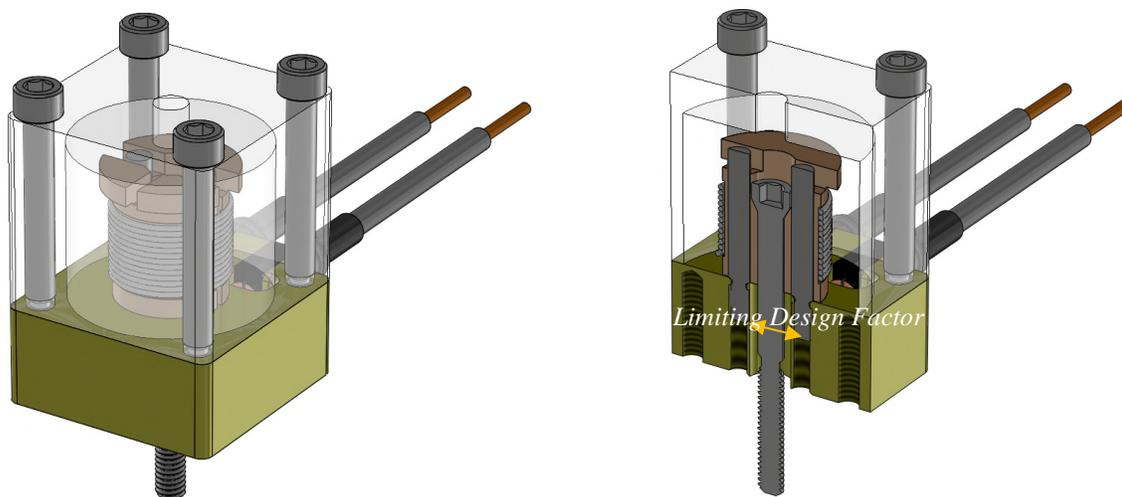
*Figure 5. Release Rod and Release Mechanism Modified*
