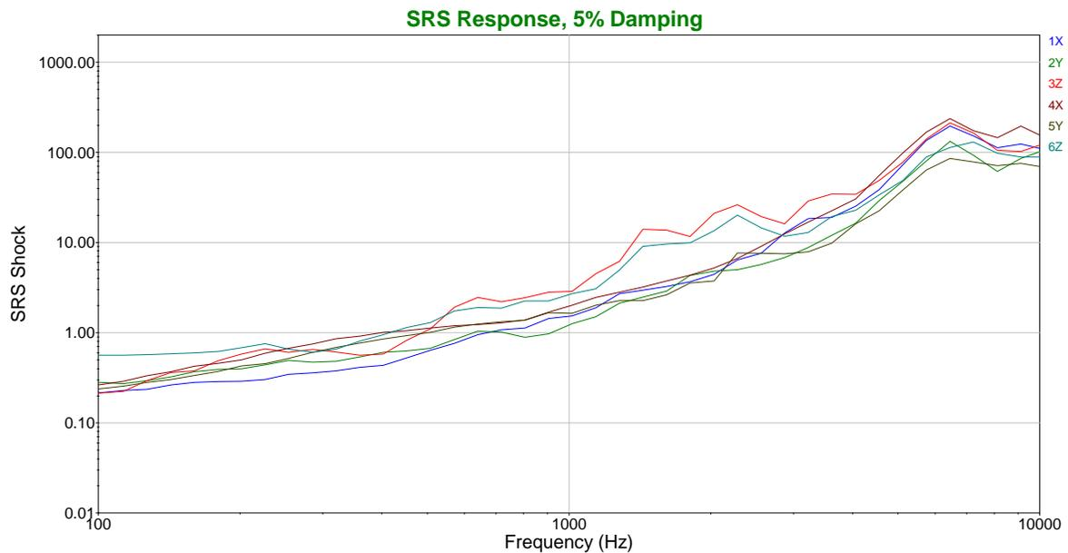
Figure 8. Shock Output Test Results
