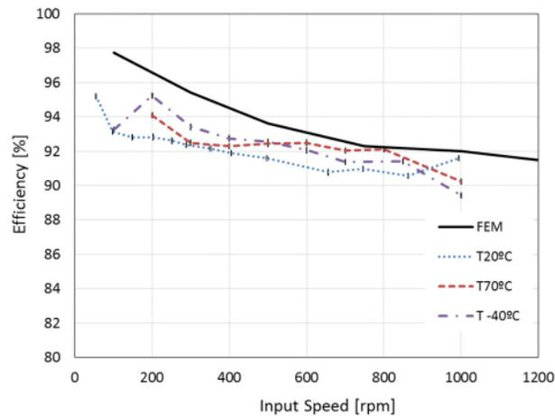
Figure 7. Efficiency test results at different temperatures
