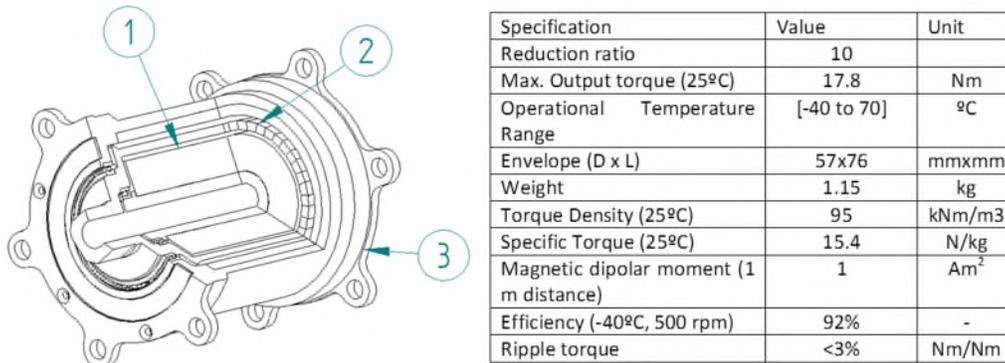
Figure 2. Assembled gearbox and summary characteristics
