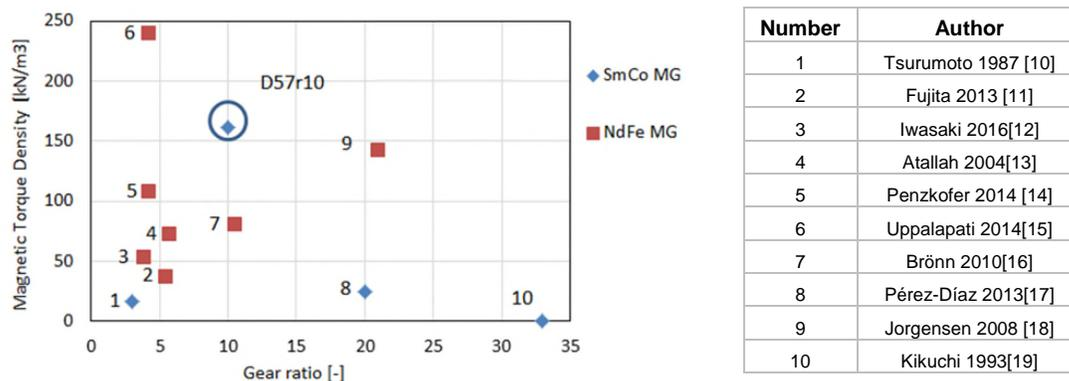
Figure 1. Summary of the state of the art of Magnetic Gearboxes
