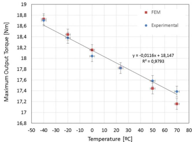
Figure 4. Maximum output torque vs temperature characterization
