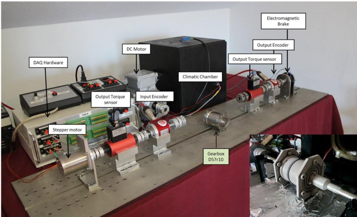
Figure 3. Dedicated test bench and a view of frozen model after -40°C test
