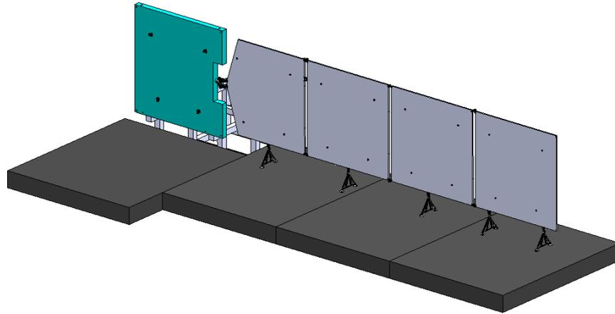
*Figure 12. Using air pad for ground testing*
