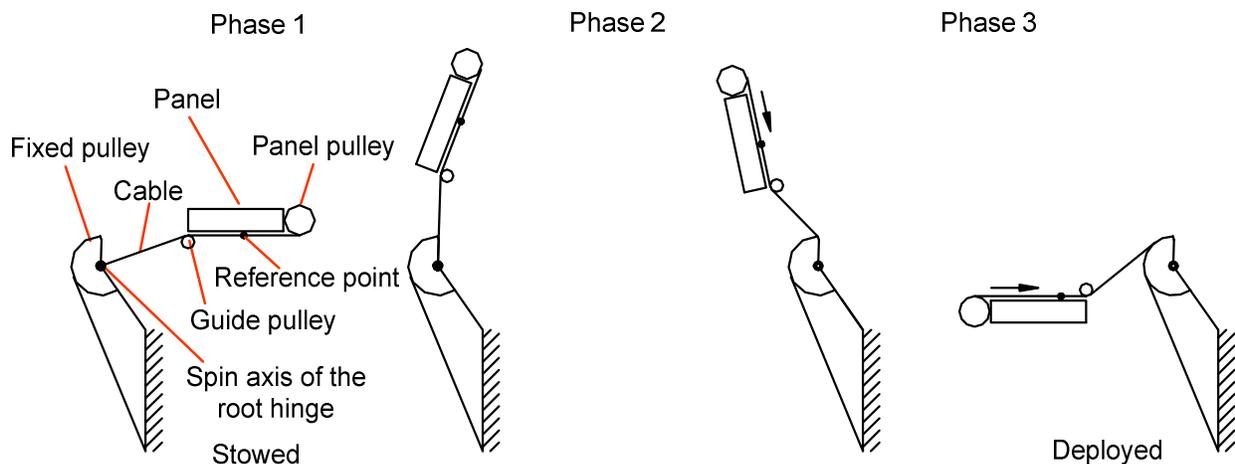
Figure 3. The schematic of fixed pulley and cable
