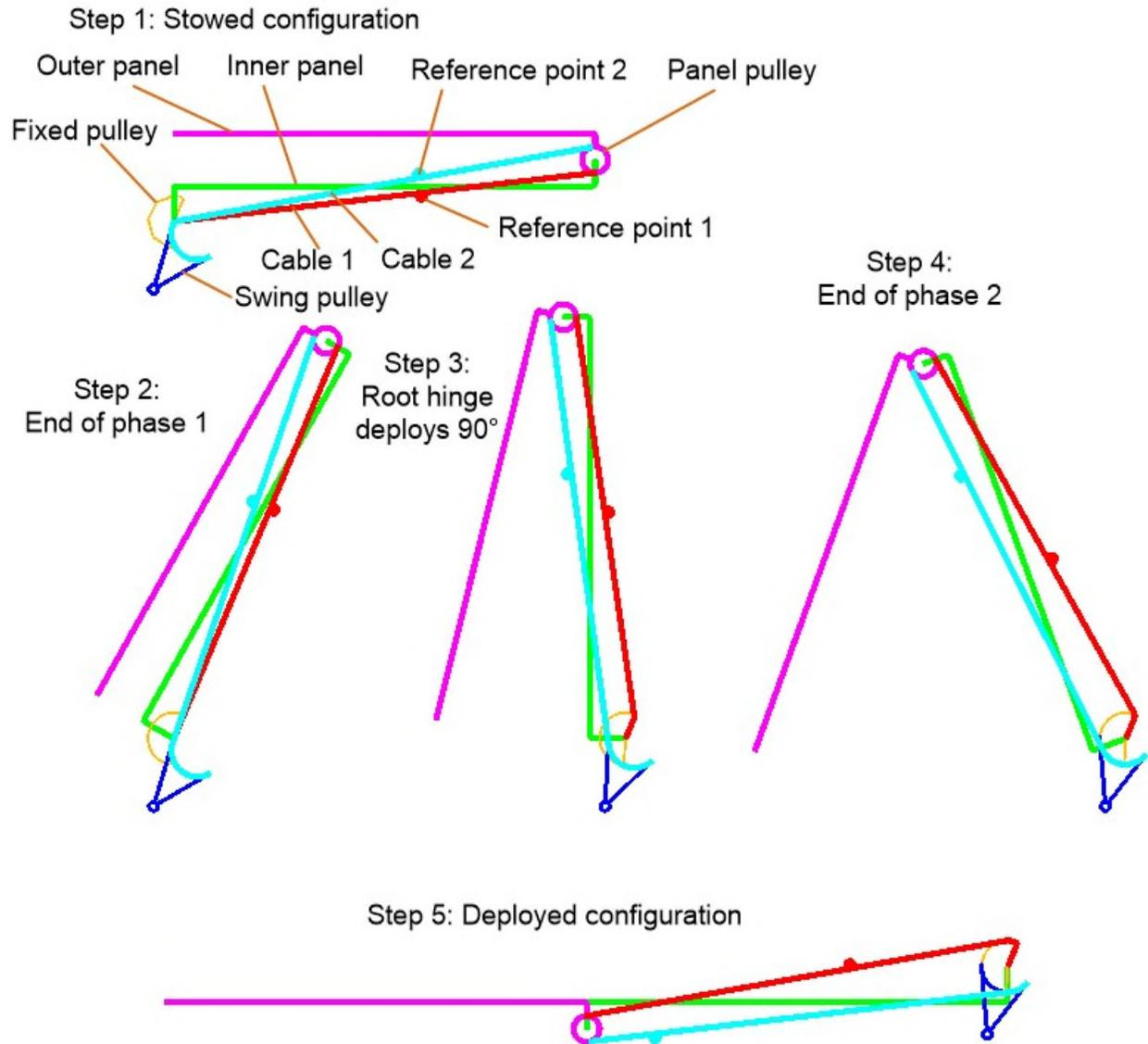
Figure 5. Deployment of solar array
