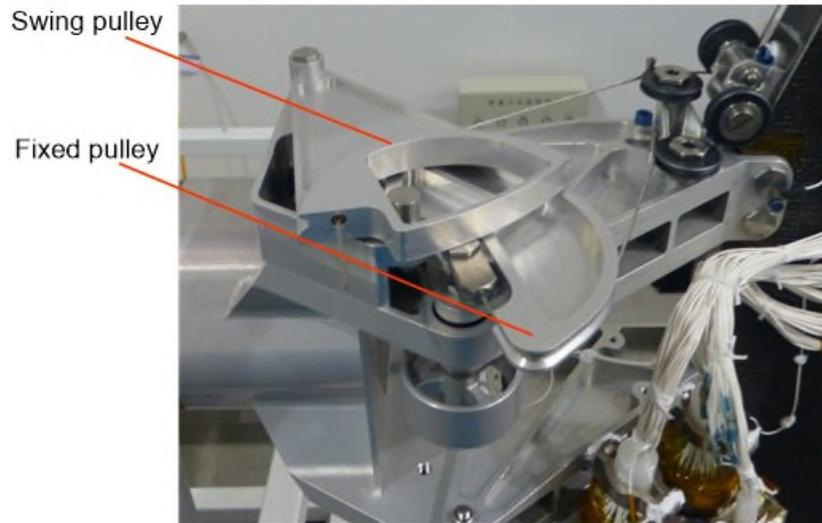
Figure 10. Deployed configuration of root hinge
