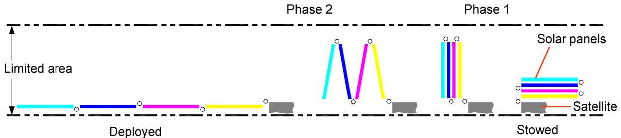
Figure 1. The two-stage deployment
