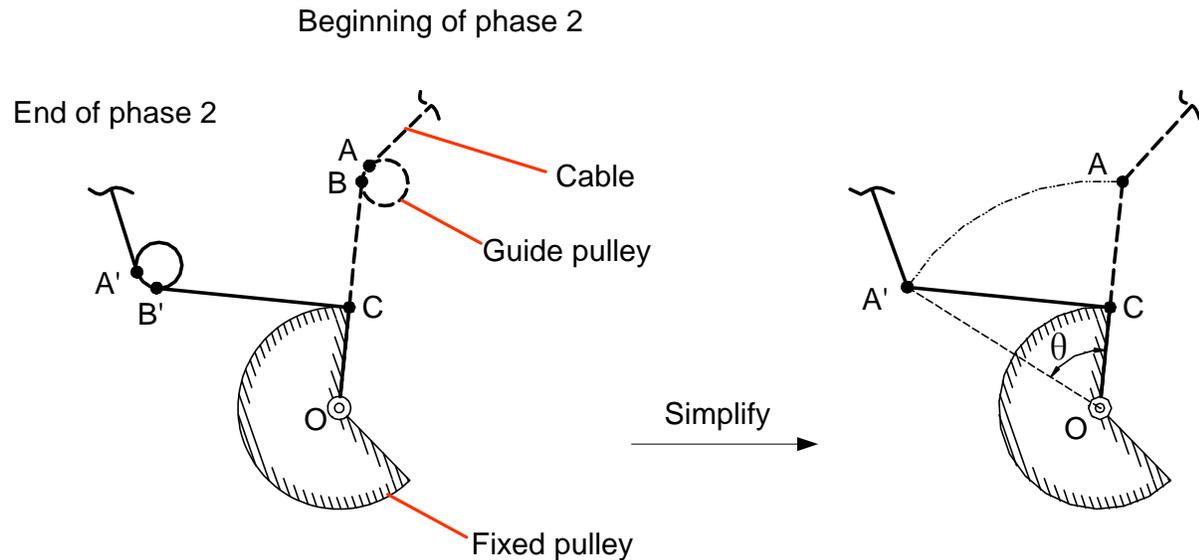
Figure 6. Mathematical model of the fixed pulley
