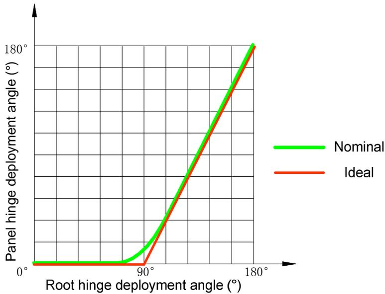
Figure 9. The synchronization characteristic
