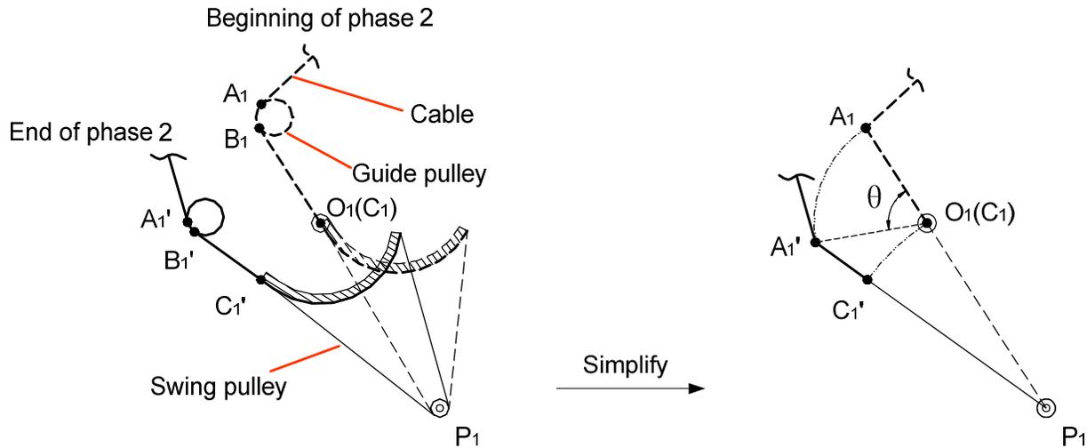
Figure 7. Mathematical model of the swing pulley
