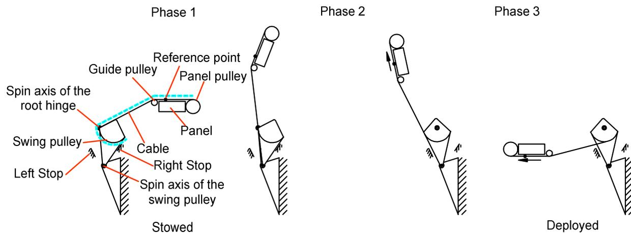
Figure 4. The schematic of swing pulley and cable
