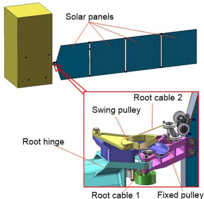
Figure 2. The root pulley of GF-3 solar array
