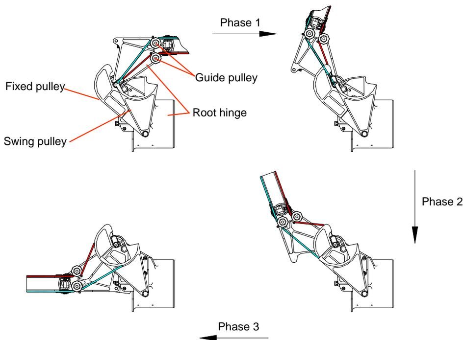
Figure 11. The three-stage deployment of root hinge
