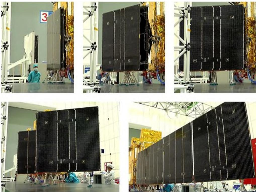
*Figure 13. The deployment of the flight model*
