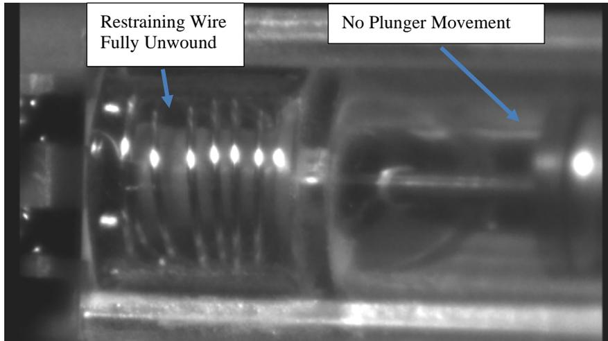
Figure 3: Unwound Restraining Wire with No Movement
