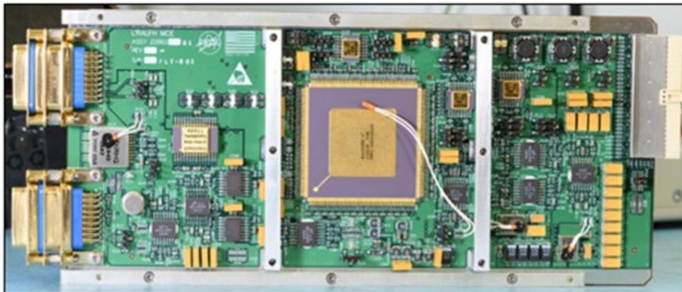
*Figure 14. L'Ralph Flight Mechanism Control Electronics*
