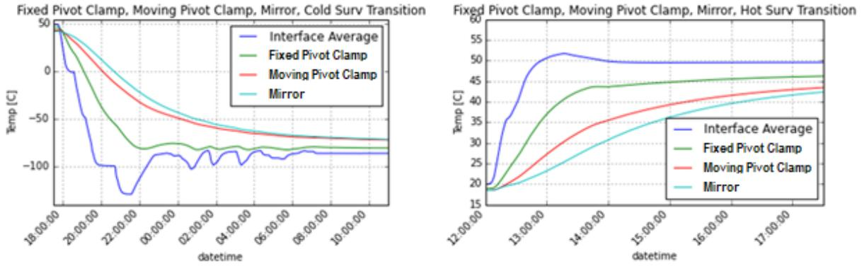
Figure 10. Fixed Pivot Clamp, Moving Pivot Clamp, and Mirror Temperature Transitions
