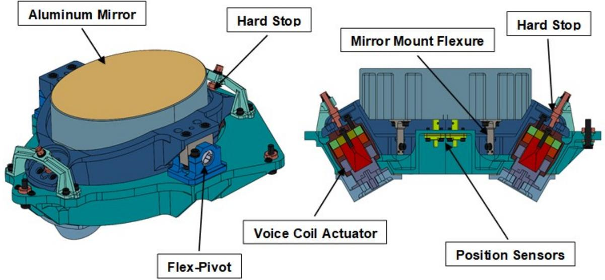
Figure 2. New Development L'Ralp Scan Mirror Mechanism
