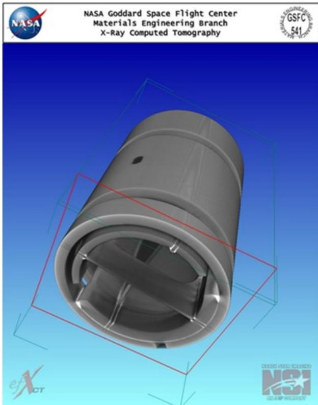
Figure 8. Flex Pivot X-Ray Cross-Section
