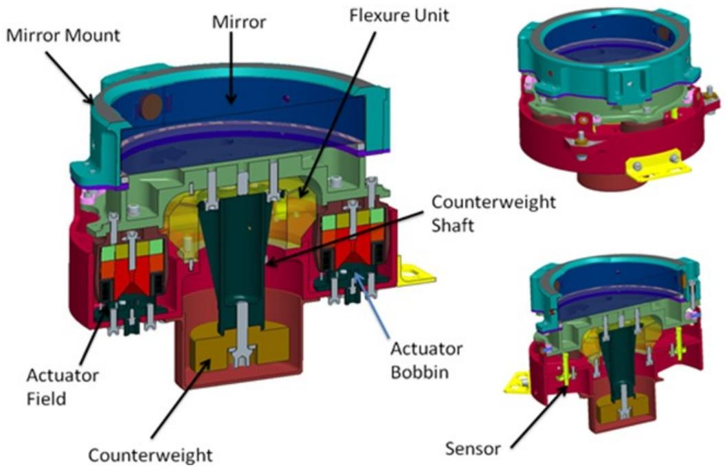
Figure 1. Previous Development ATLAS Beam Steering Mechanism
