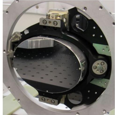
Figure 15. L'Ralph Flight Scan Mirror Mechanism Front View
