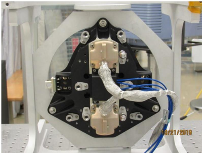
Figure 16. L'Ralph Flight Scan Mirror Mechanism Rear View
