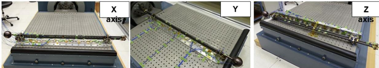
Figure 5. Configuration of LP-PWI on the shaker
