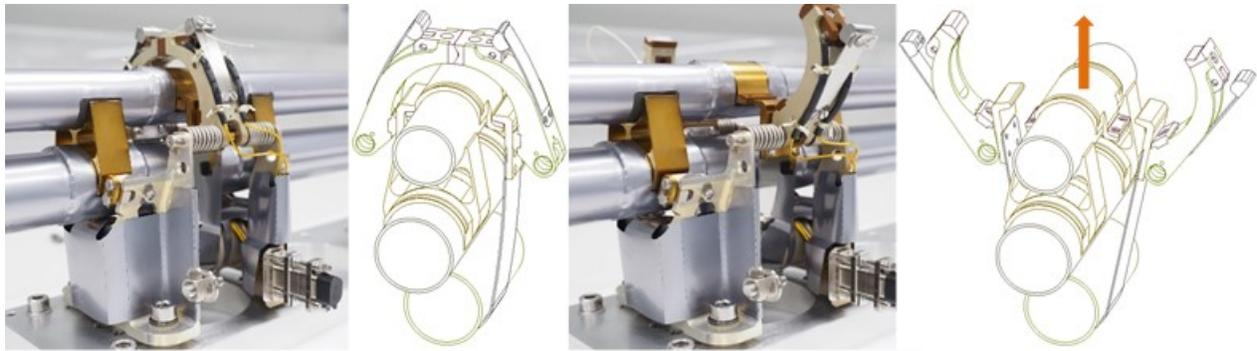
Figure 3. Closed HDRM #2 - left; Open HDRM #2 - right
