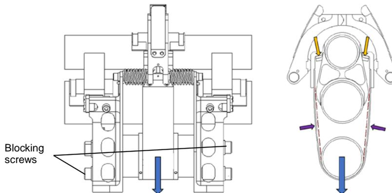
Figure 4. Application of the preload in HDRM
