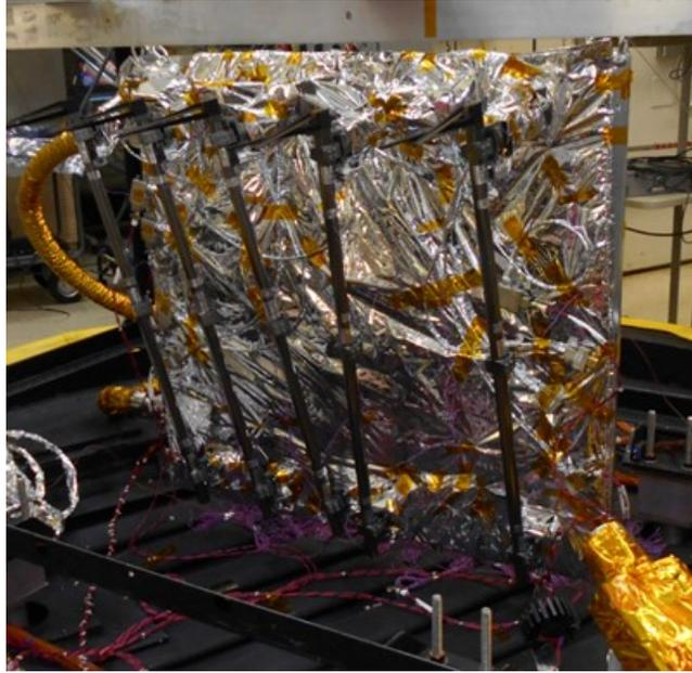
Figure 9: Flight clamshell mechanisms staged for TVAC testing.
