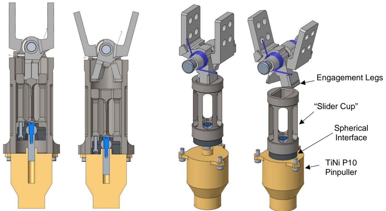
Figure 5: The details of the active clamshell hinge, in stowed and deployed positions.
