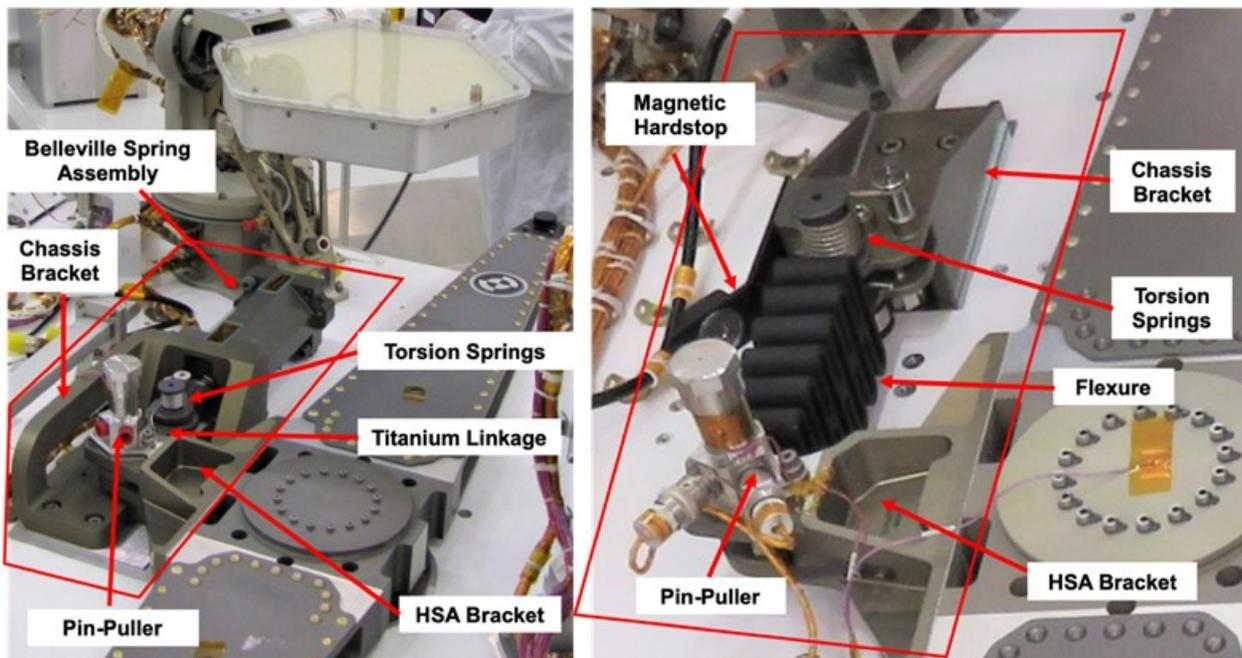
Figure 2: MSL CDPR (left) versus Mars 2020 CDPR (right)
