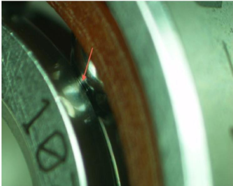
*Figure 2. Oil meniscus present in R4 Bearing after 7% lubricant slosh (Nye Synthetic Oil 2001/heptane).*
