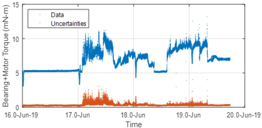
Figure 6. Motor 33 torque signature for dry cage instability.
