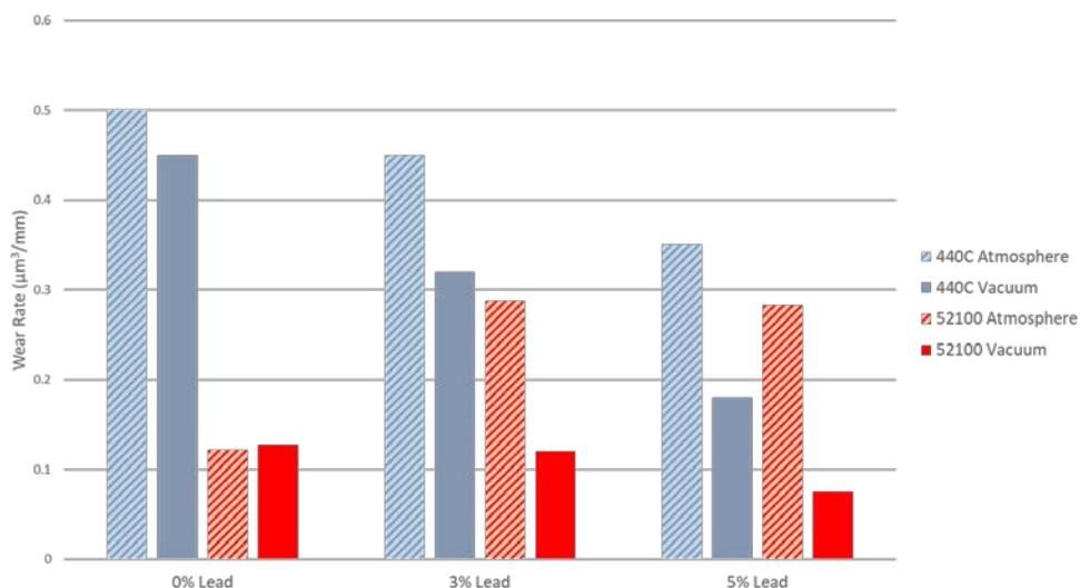
*Figure 5: Boundary Lubrication Wear Rate at 75°C*
