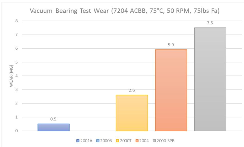
Figure 10: Vacuum Bearing Wear Test on Greases
