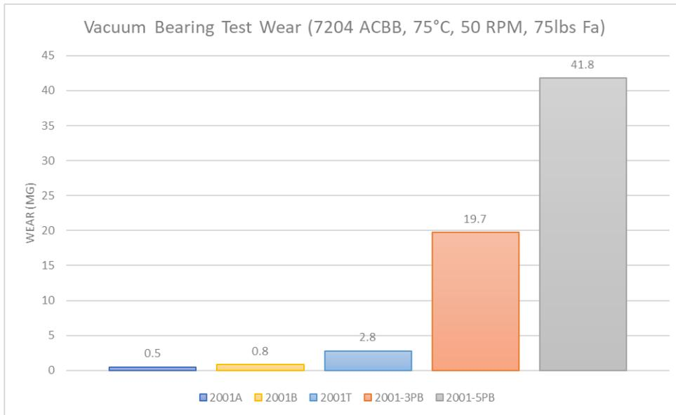
Figure 9: Vacuum Bearing Wear Test on Oils
