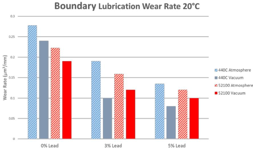
Figure 4: Boundary Lubrication Wear Rate at 20°C
