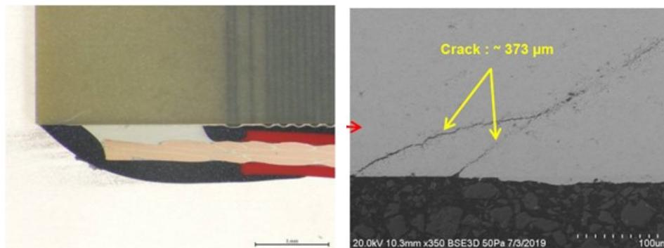
Figure 5. Solder Inspection, Example of a Crack
