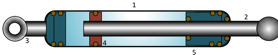
*Figure 3. COTS Gas Spring Actuator Schematic*
