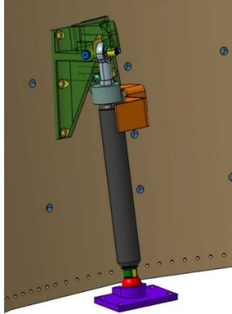
*Figure 4: Actuator I/F schematic*
