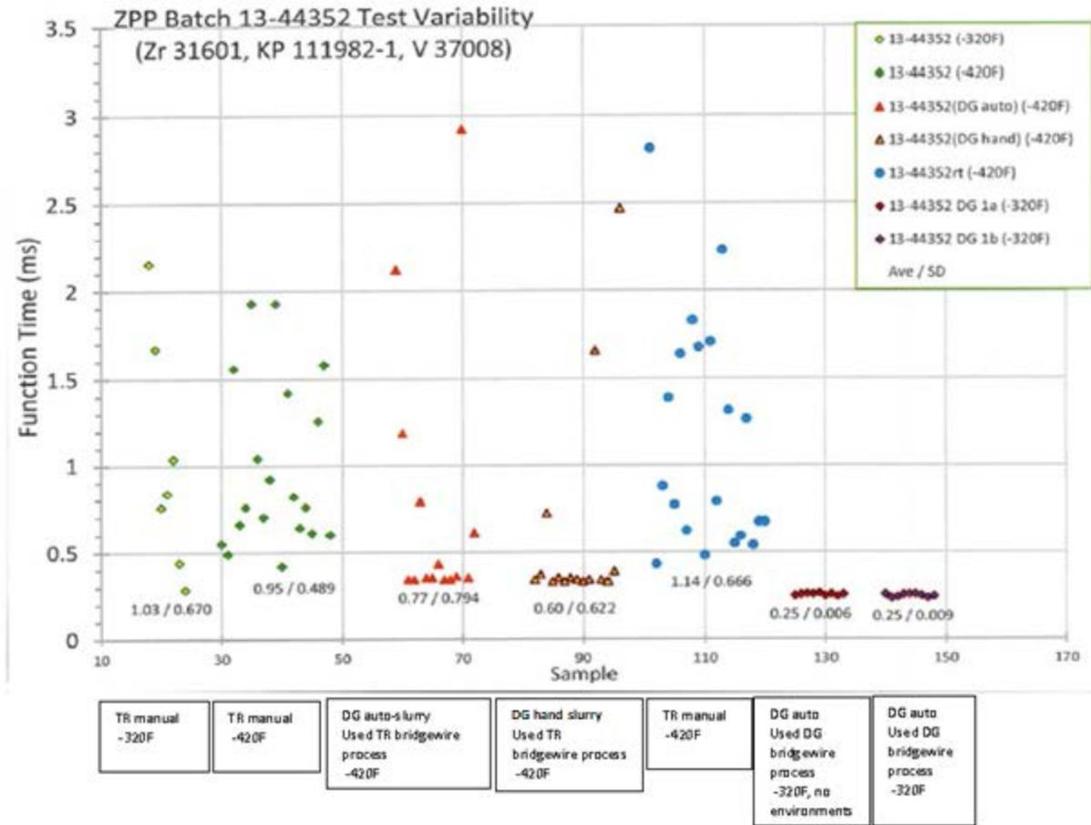
Figure 4. Effect of Process Automation on ZPP L/N 13-44352
