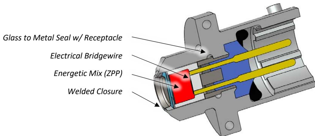
Figure 1. Cross Section of NASA Standard Initiator (NSI)
