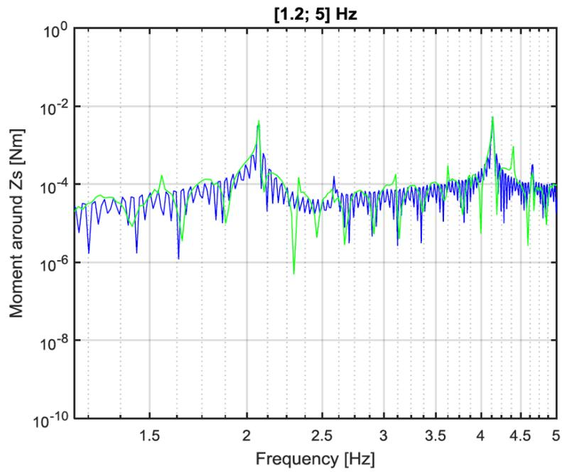
Figure 14. Simulated (blue) vs measured (green)  $\mu$ Vib
