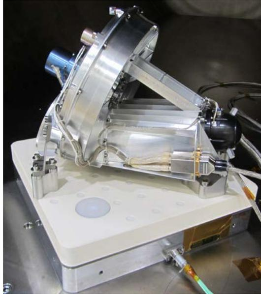
Figure 12. UVN CAA mounted on  $\mu$ Vib table
