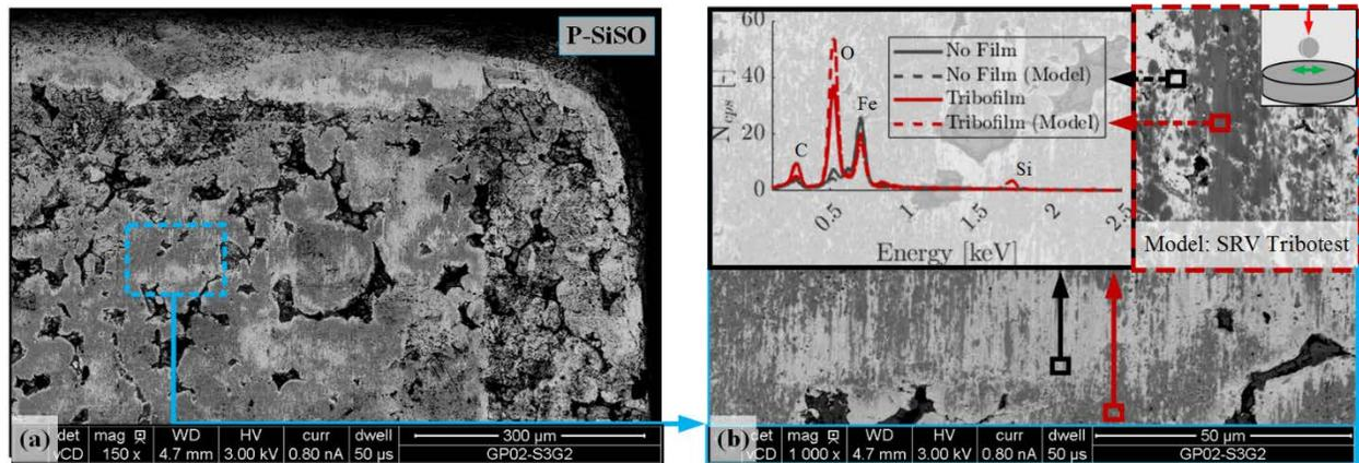
Figure 6. SEM-EDS analysis of P-SiSO driven gear Region II. (a) Overview indicate gear surface is covered with tribofilm. (b) Gear tribofilm compared to P-SiSO tribofilm generated in ball-on-flat SRV tribotest.
