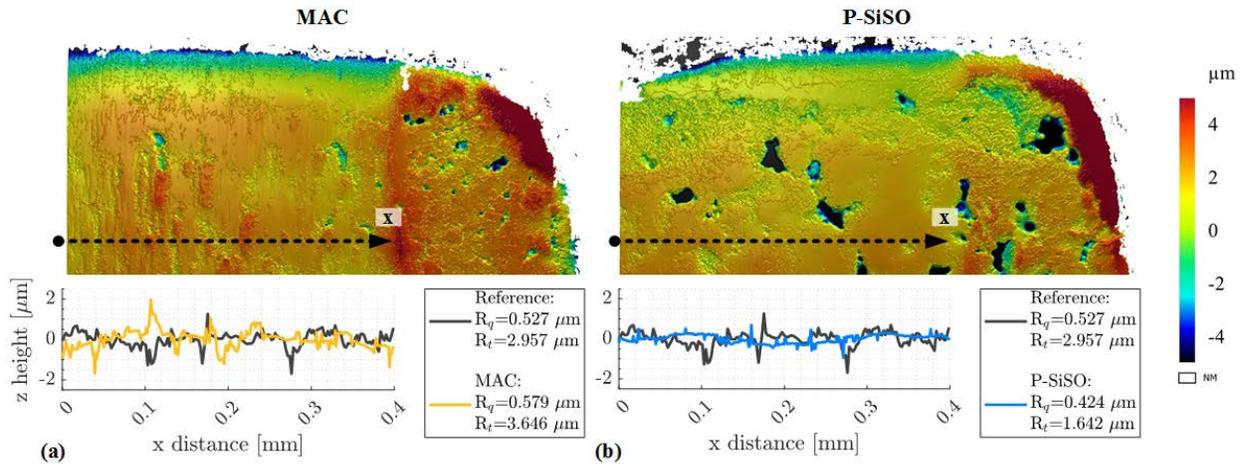
Figure 5. Regions I-II of MAC and P-SiSO respectively, with roughness profiles and parameters along  $x$  profile. (a) MAC surface show evidence of partial seizures (scuffing). (b) P-SiSO produce smooth contact patches and retains the porous structure of the unworn sintered material.
