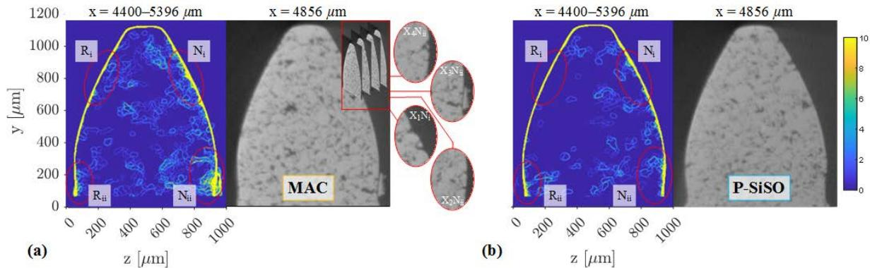
Figure 7. XMT analysis indicates potential sub-surface cracking. Driven side dedendum ( $N_{ii}$ ) is critical region. (a) MAC show severe scuffing with large particles adhered at  $N_{ii}$ , and evidence of subsurface cracks in the same region (b) P-SiSO show less overall detected edges, and no evidence of scuffing.
