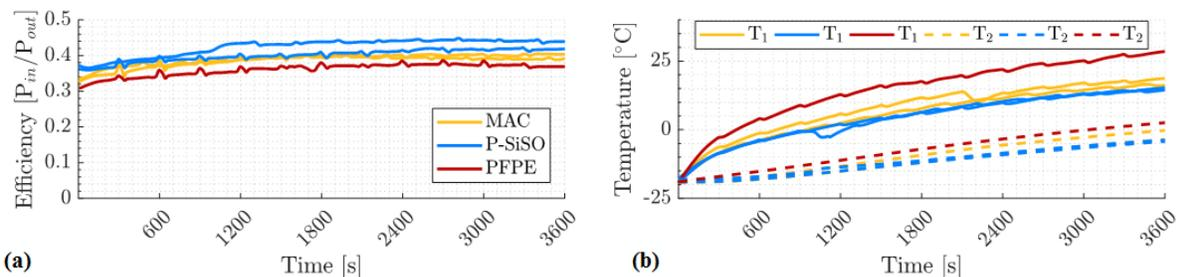
Figure 2. (a) Measured efficiency of actuator setup when lubricated with MAC, P-SiSO, and PFPE respectively. lubricants. (b) Gearbox housing temperature ( $T_1$ ) and chamber interior temperature ( $T_2$ ) over 1 h test (500 000 input revolutions). As expected, efficiency is inversely related to increasing gear house temperature ( $T_2$ ).
