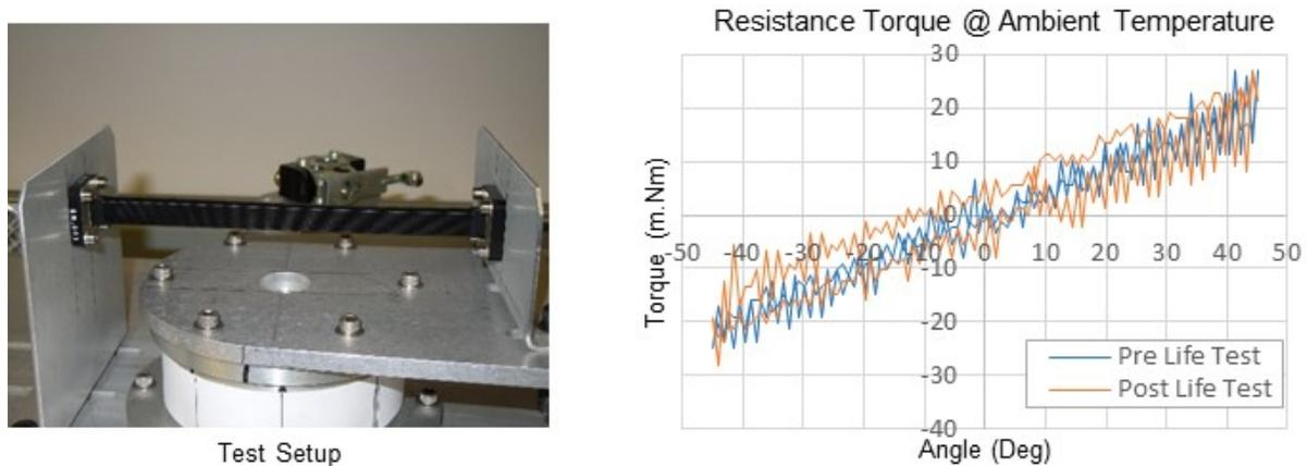
*Figure 3. Resistance Torque and Life Cycle Test*
