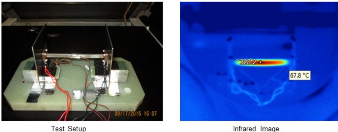
*Figure 8. RF Induced Waveguide Heating - Measurement*
