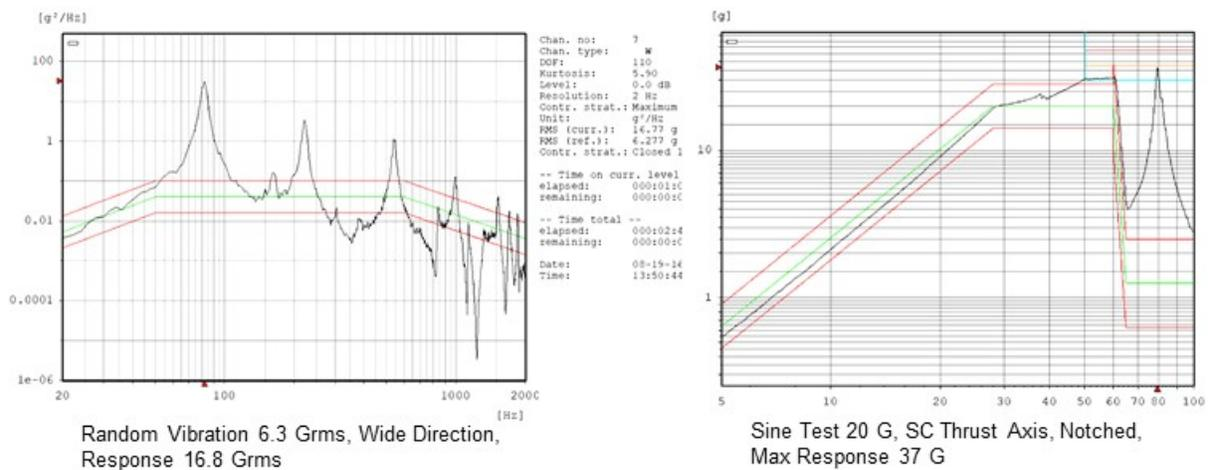
Figure 6. Vibration Test Responses
