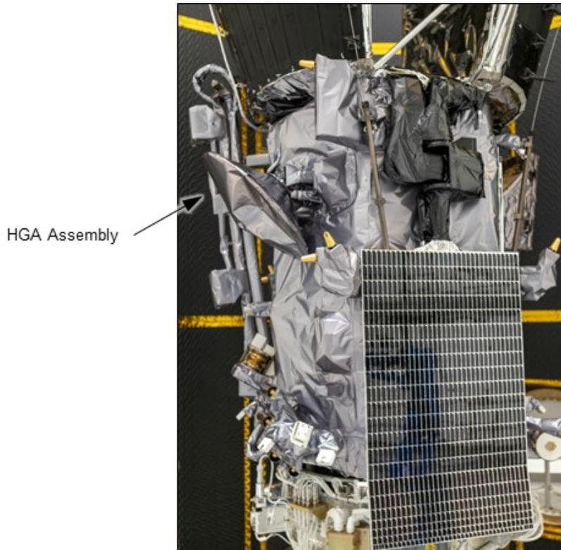
*Figure 16. HGA Assembly on PSP Spacecraft*
