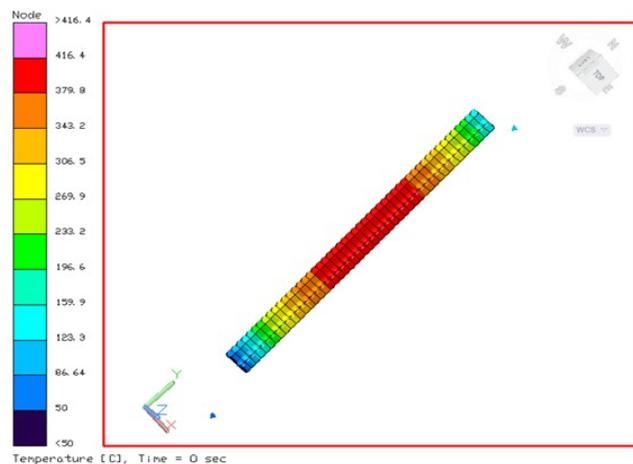
*Figure 7. RF Induced Waveguide Temperature - Prediction*
