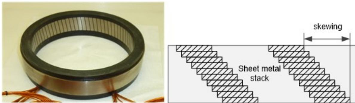
Figure 5. Motor stator skewing
