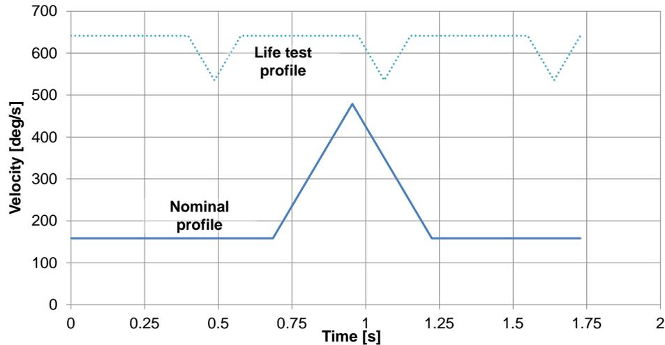
Figure 13. Scanner life test profile for acceleration factor 3
