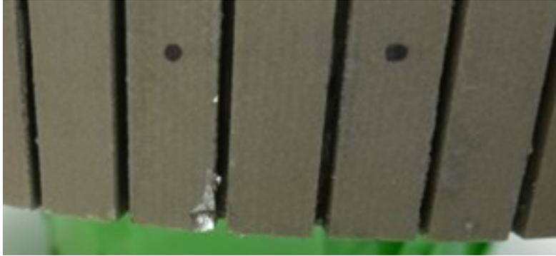
Figure 11. SmCo magnets damaged during AIT
