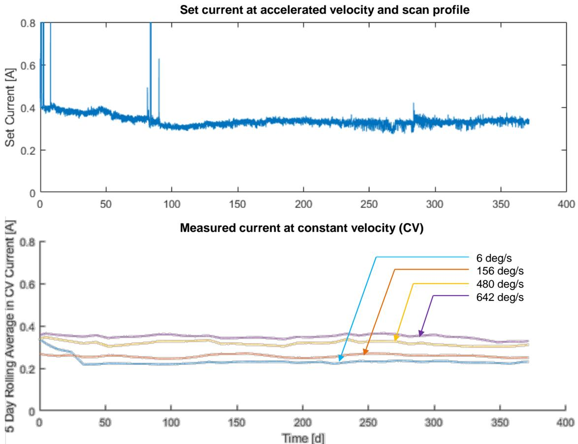
Figure 14. Scanner motor current during first 55 million revolutions
