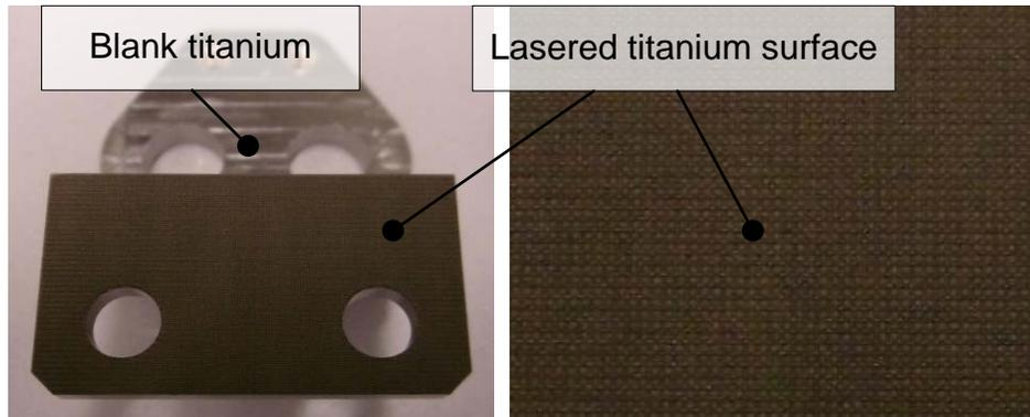
Figure 9. Laser-modified surfaces for increased friction coefficient
