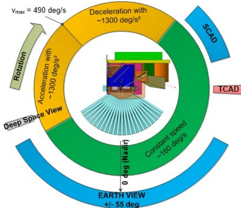
Figure 6. Scan profile of Scanner and Derotator
