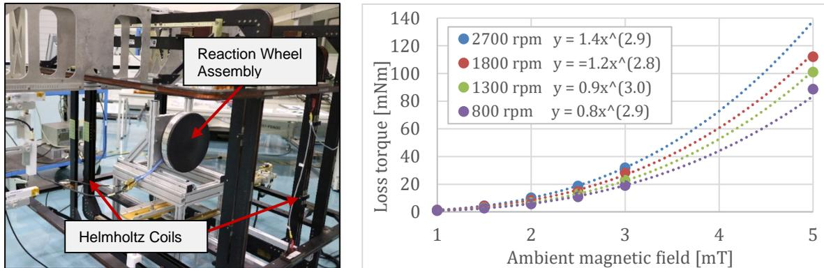
Figure 6 - Left: Test configuration (reaction wheel spin axis orthogonal to the magnetic field vector)
