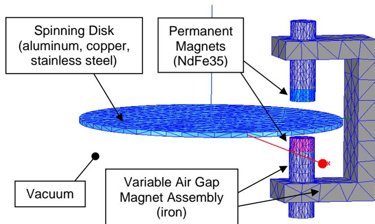
Figure 1 – Model configuration & mesh in ANSYS Maxwell®
