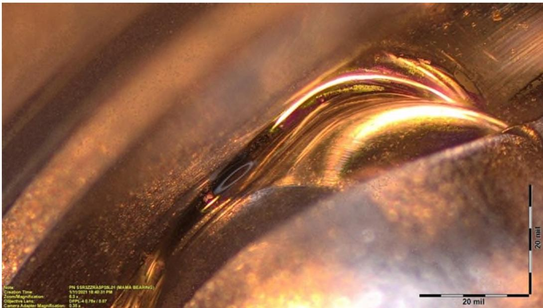
*Figure 2. Microscopic View of Bearing Showing Oil Meniscus*
