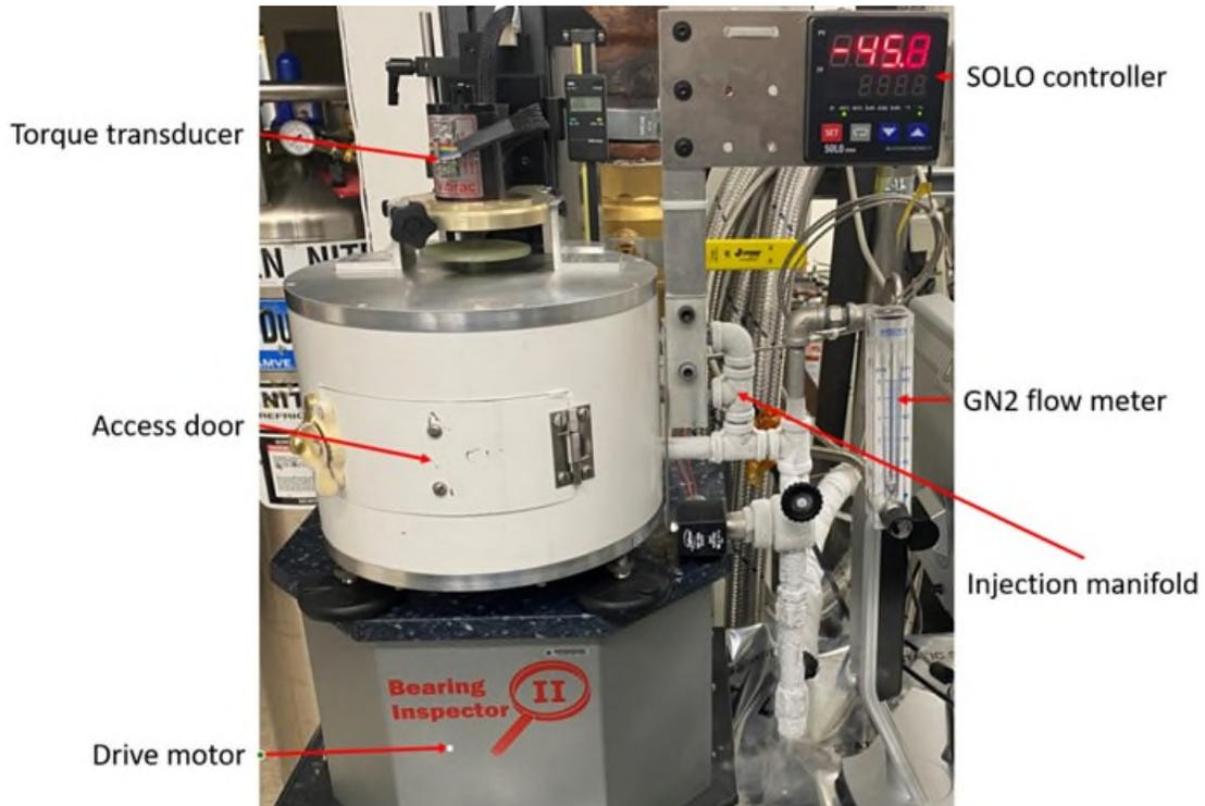
Figure 3. Test Apparatus
