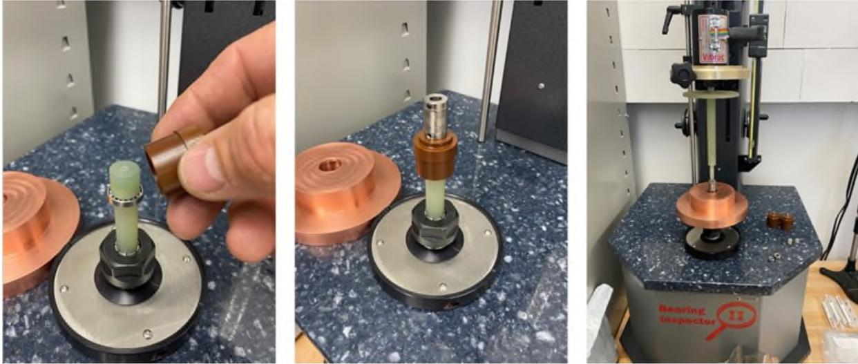
Figure 6. Bearing Support and Connection to Torque Tester
