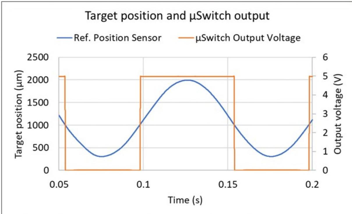
Figure 12. Sensing Test Results – Proximity Detection
