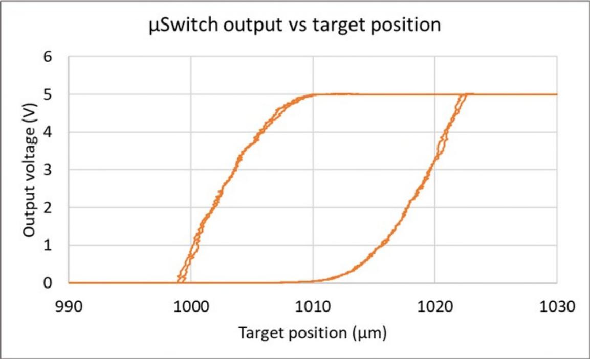
Figure 13. Sensing test results – Forward / backward hysteresis threshold
