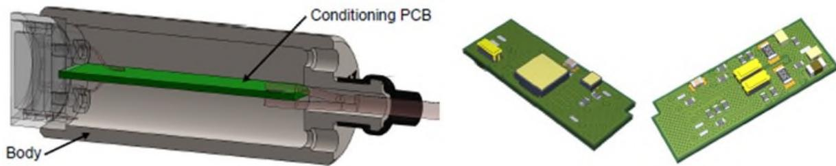
Figure 6. Micro-switch embedded space-grade conditioning PCB design
