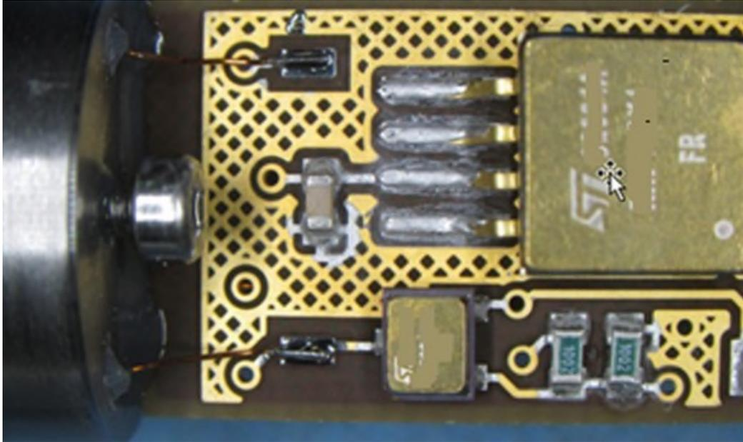
Figure 9. Space Grade EQM Embedded Conditioning Electronics
