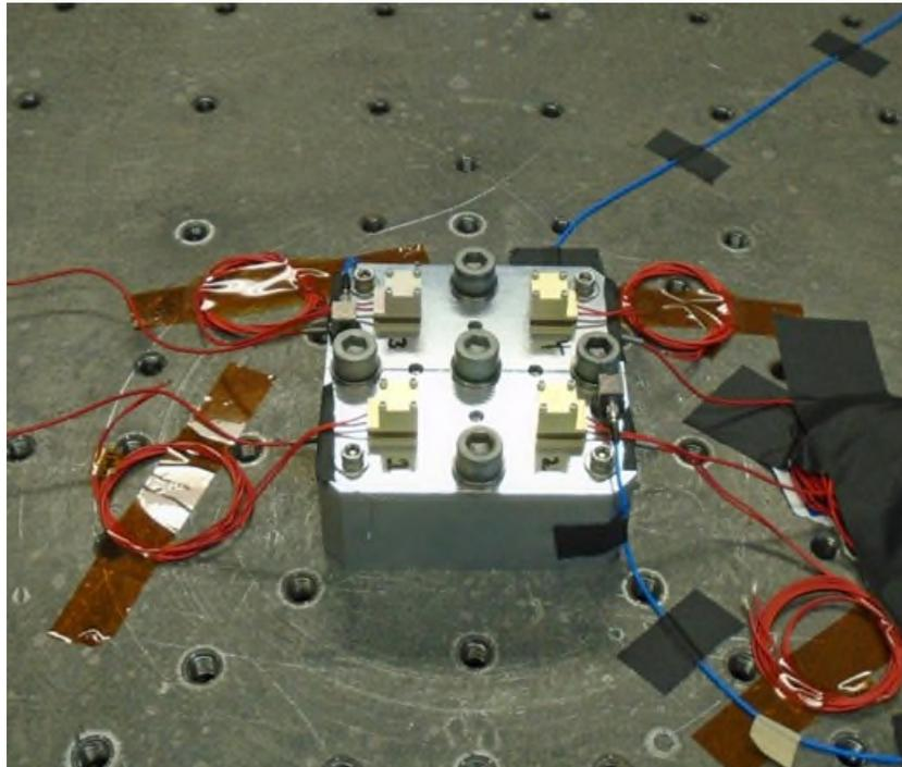
*Figure 6. Mini HDRM Random Vibration Test Setup*
