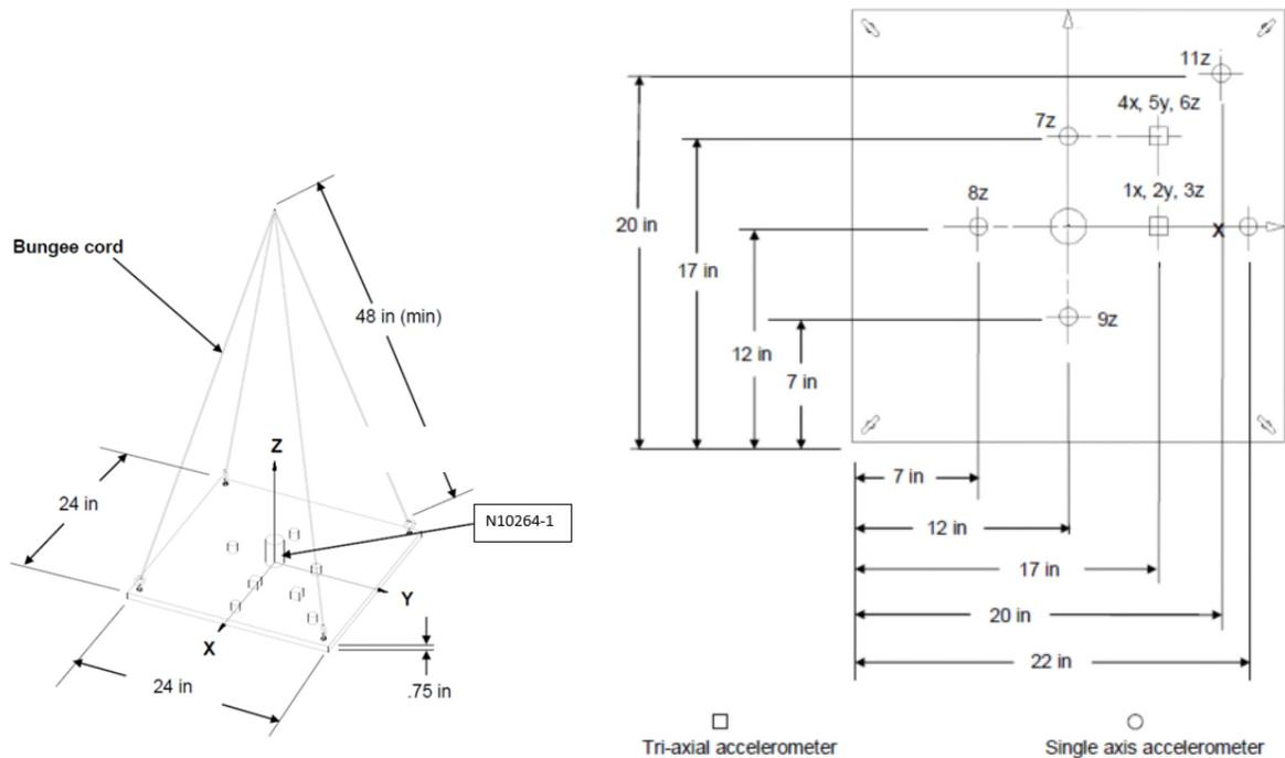
Figure 12. Mini HDRM Output Shock Test Setup Parameters
