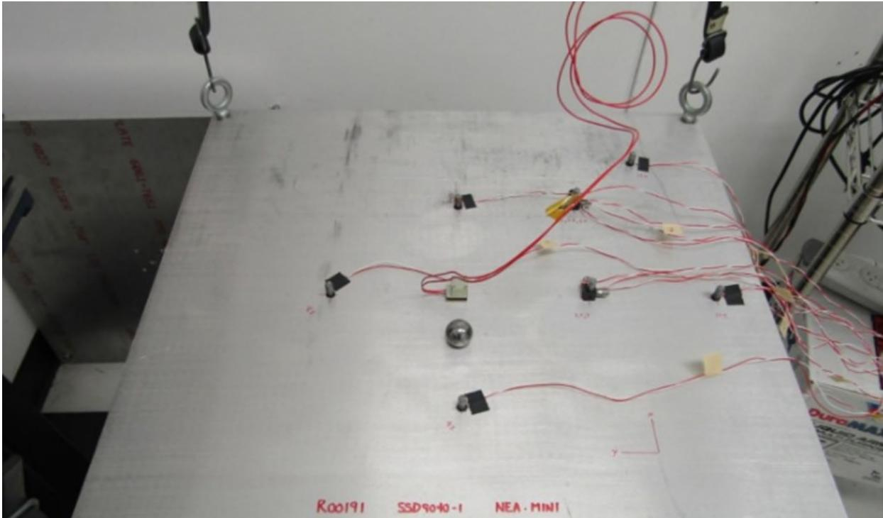
Figure 13. Mini HDRM Output Shock Test Setup Photo
