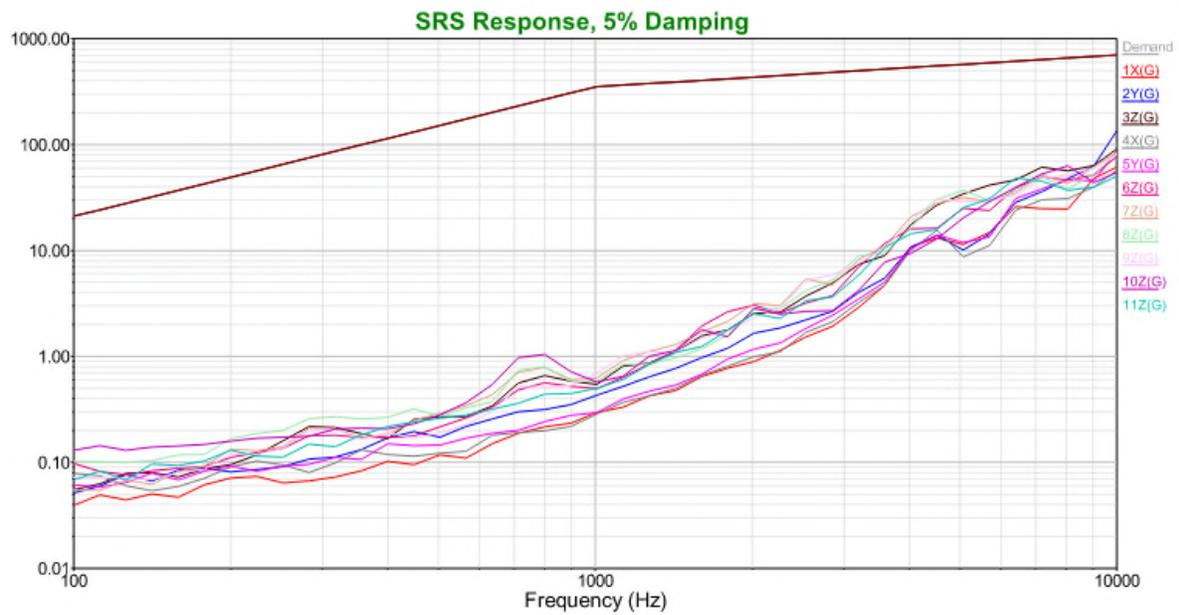
Figure 14. Mini HDRM Output Shock Test Results
