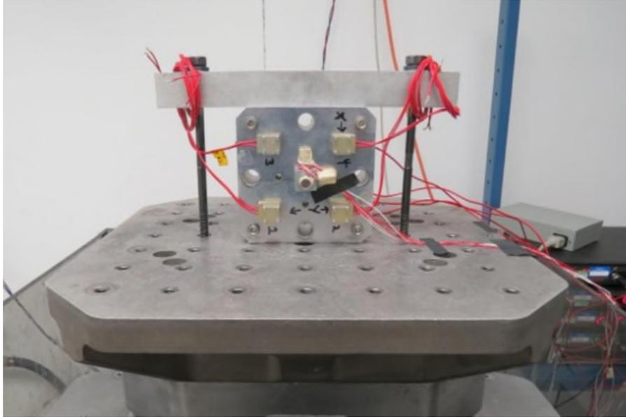
Figure 8. Mini HDRM Input Shock Test Setup
