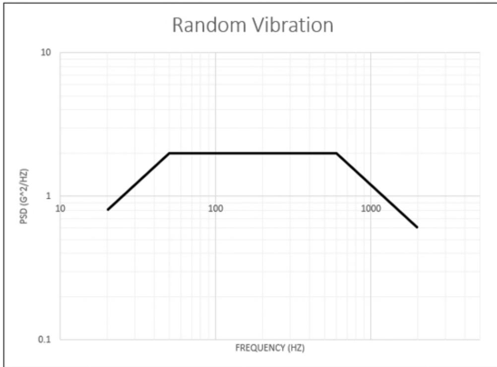
Figure 7. Mini HDRM Random Vibration Test Parameters
