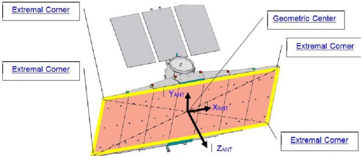
Figure 2. SAR Antenna OARP and coordinate system.
