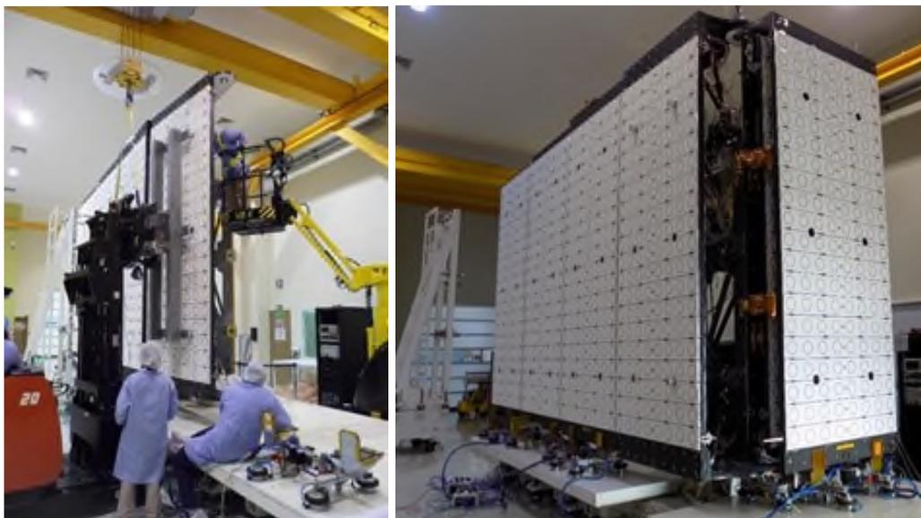
*Figure 8. SAR Antenna during integration in vertical position, one panel at the time.*
