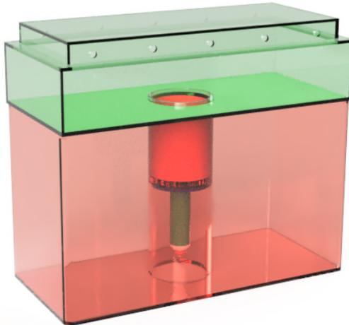
*Figure 1. Rendered image showing layout of current GMPE design. The fuel tank is the red region, the electronics compartment and satellite bus interface are at the green region, and the thruster can be seen in the center of the module.*
