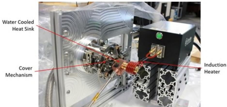
*Figure 10: NEG activation and heat sink. NEG activation involved an induction heater heating the NEG pumps to 500°C. A water cooled heat sink was mounted to the NEG seal to prevent damage to the critical sealing interface. Credit: Sierra Space Corporation*
