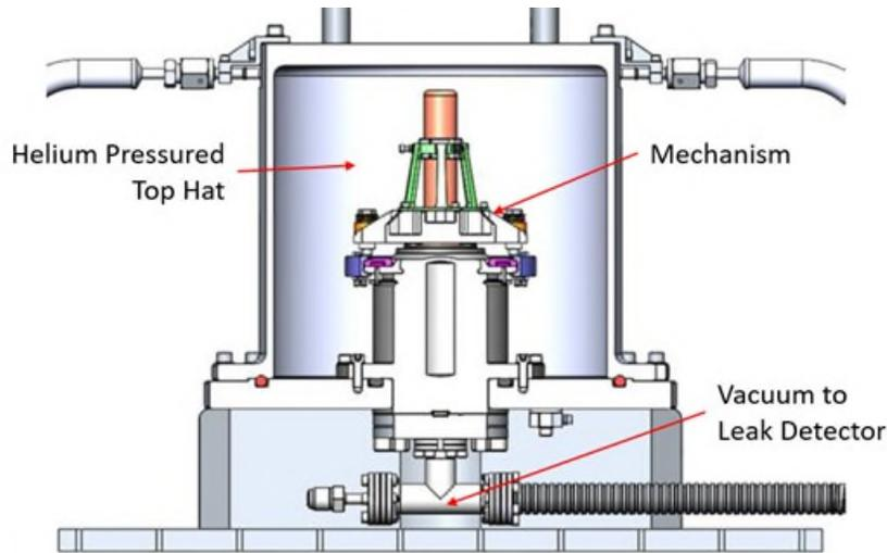
*Figure 11: Leak chamber for cover mechanism. Helium was backfilled into a top hat, with a leak detector pulling vacuum on the other side of the seal, monitoring for He leak. Credit: Sierra Space Corporation*
