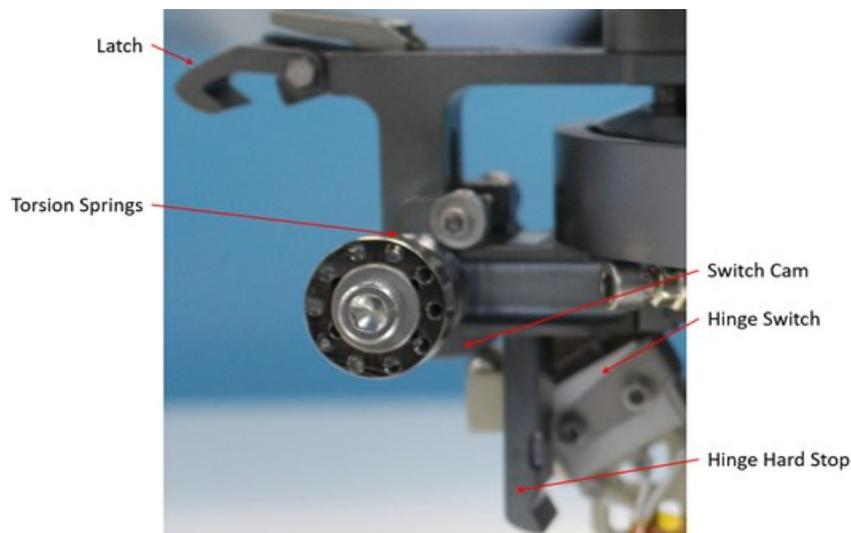
*Figure 4: Hinge and latch assembly in stowed state. Latch assembly prevents rebound of cover and locks the upper ring assembly below the instruments aperture following mechanism deployment. Credit: Sierra Space Corporation*
