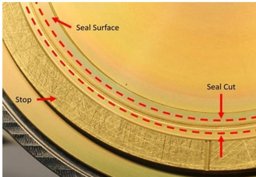
*Figure 5: Desired cut from knife-edge onto capped H-seal. Cut is concentric relative to stop and sealing surfaces. The resulting cut is clean with not nicks or blemishes. Credit: Sierra Space Corporation*
