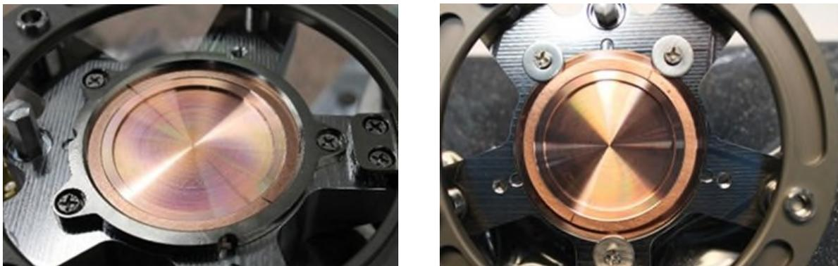
*Figure 7: (Left) Original seal retention method (Right) Updated seal retention method. The original seal retention method did not give proper clearance to the antechamber to allow for the seal to be loaded correctly, and prevented proper deployment of the cover. Credit: Sierra Space Corporation*
