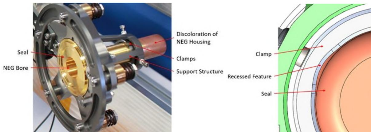
*Figure 9: (Left) NEG Seal following activation with support fixture installed. The support fixture was required to prevent deflection of the NEG pump seal housing. The NEG seal was discolored following activation where it was heated to 500°C for over 10 minutes. (Right) Clamp interface onto seal. Cut in clamp ensures two lines of contact on seal to limit Hertzian stresses. Credit: Sierra Space Corporation*
