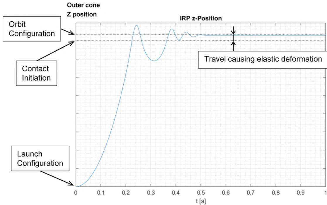
Figure 9: Configuration change travel (axial direction).
