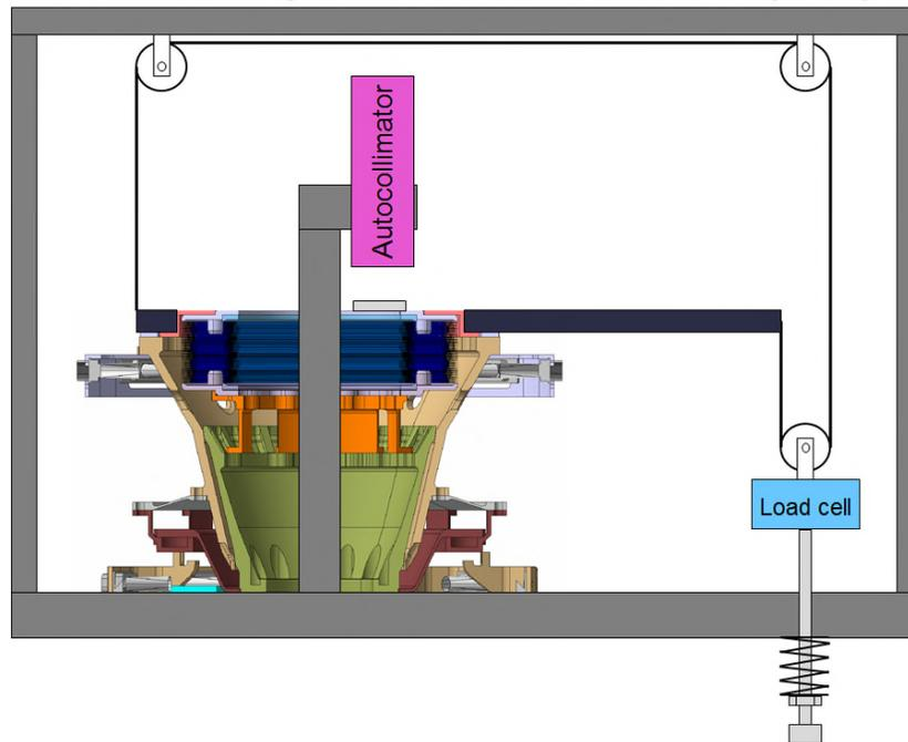
Figure 13: X-Y LOD angular stiffness, static measurement.
