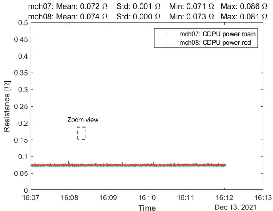
Figure 15: PDTD Resistance noise with 25 kHz sampling rate
