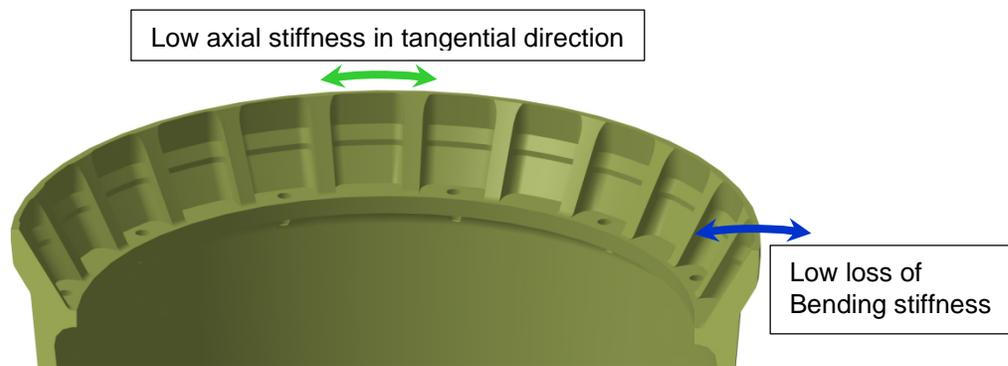
*Figure 7: Cone contacts local stiffnesses.*
