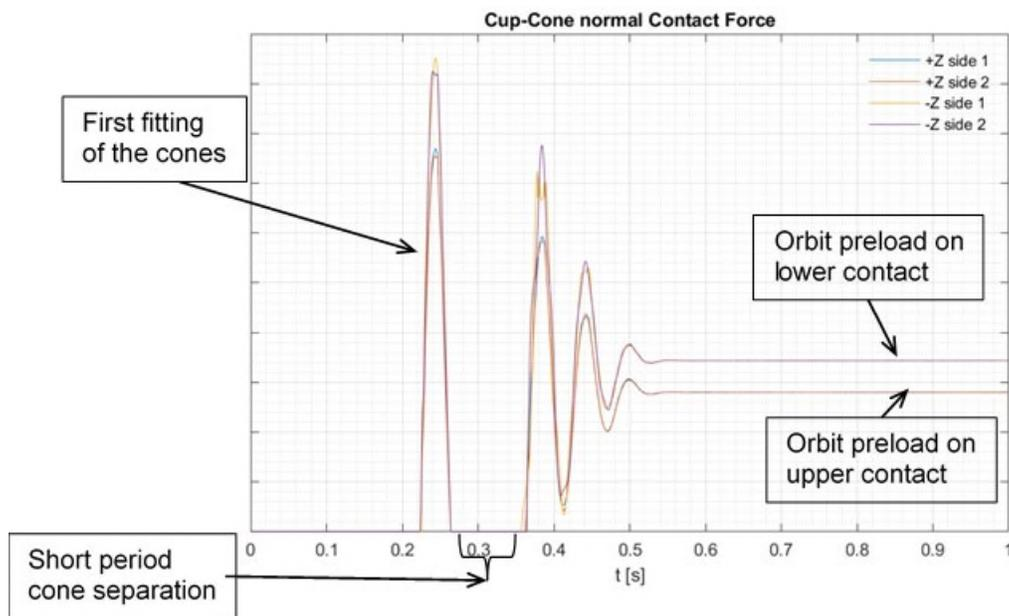
Figure 10: Contacts normal force during configuration change.
