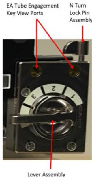
Figure 8. CIAS RHS EA Selector Mechanism Assembly
