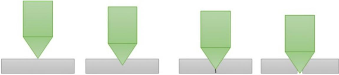
Figure 3. Illustration of Cutting Depth Leading to Uncontrolled Crack Propagation
