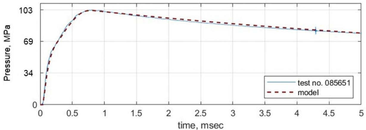
Figure 6. 2-cm<sup>3</sup> Closed Bomb Model Comparison
