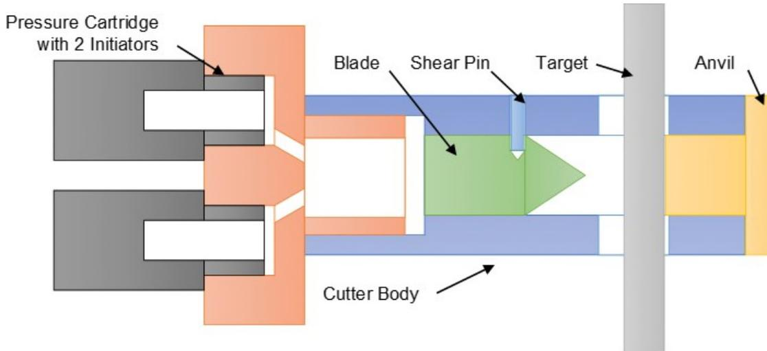
Figure 2. Conceptual Layout of Pyrotechnic Bolt Cutter
