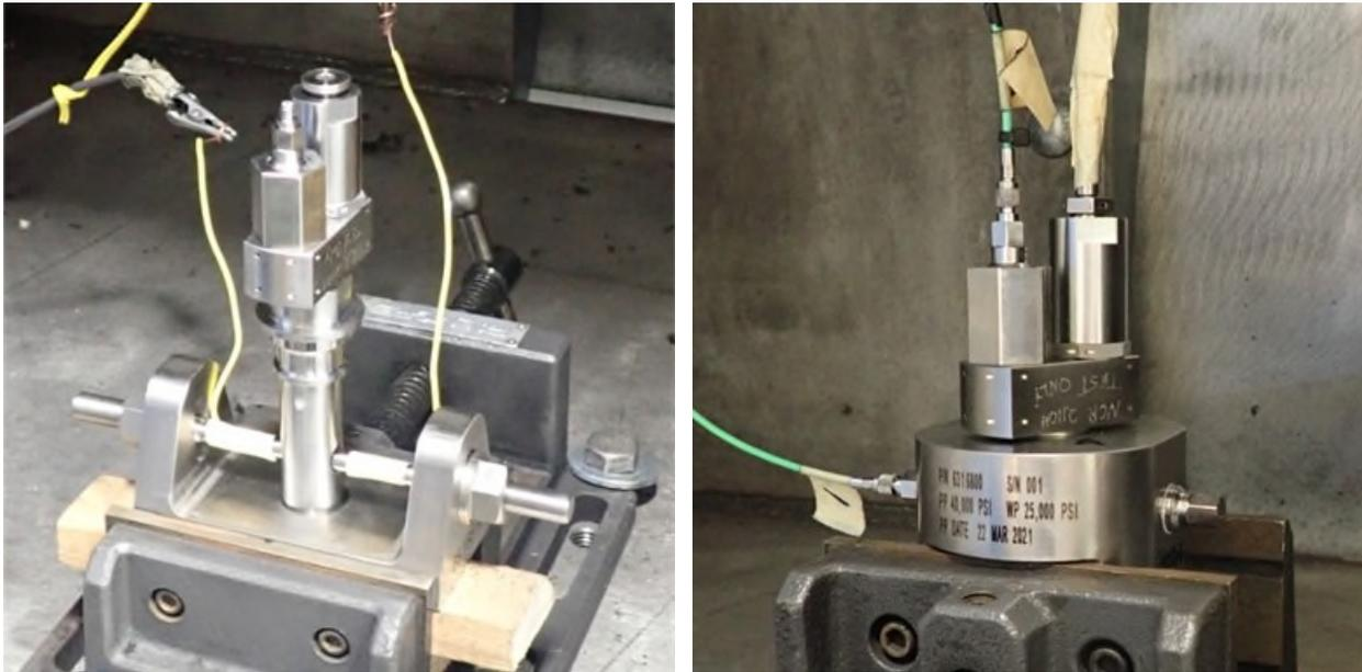
Figure 5. Functional Test Setup (left) and 2-cm<sup>3</sup> Closed Bomb (right)
