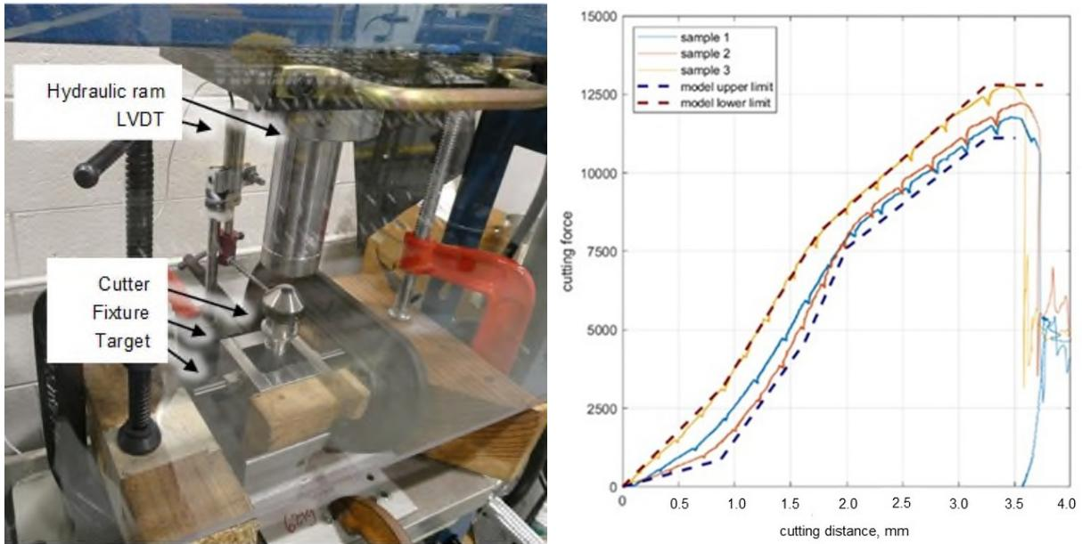
Figure 4. Cutting Force Measurement Setup (left); QS Cutting Force Model (right); Severed Target (bottom)
