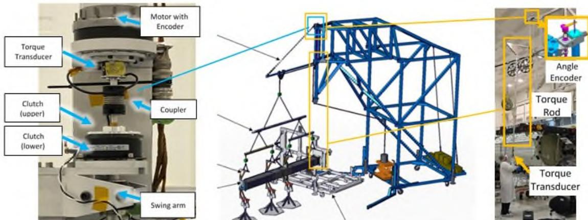
Figure 12: SWOT Motorized Torque Characterization Tool (Left), Full Swing Arm Offload System (Center), NISAR Manual Torque Characterization Tool (Right)
