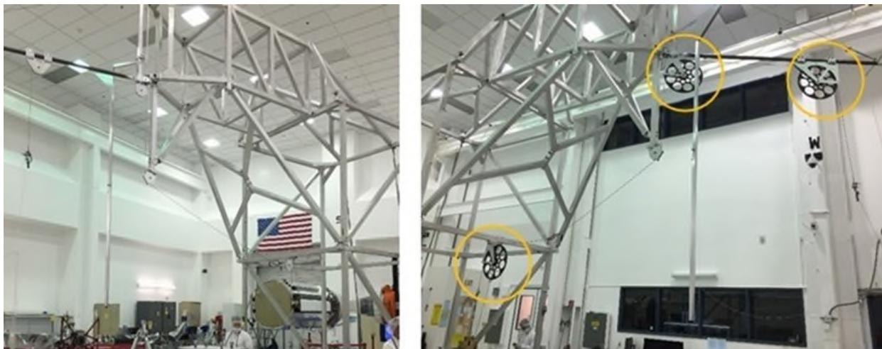
Figure 8: Deployment Fixture with 15.25-cm Diameter Pulleys Upgraded to 50.8-cm Pulleys to Reduce Drag
