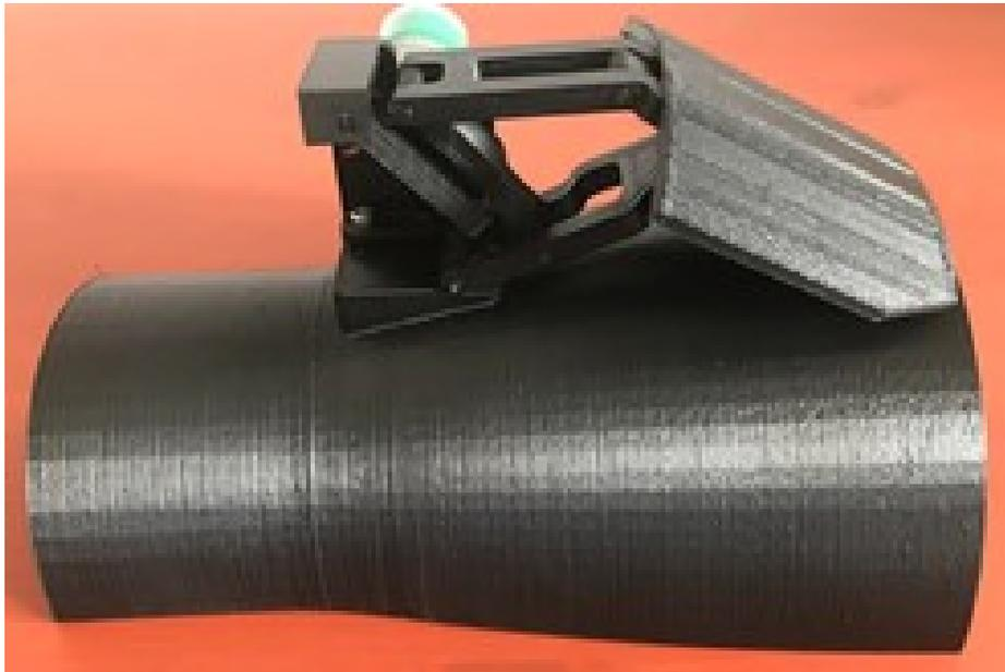
*Figure 1. Thrust Vector Control mechanism – 3D printed prototype*
