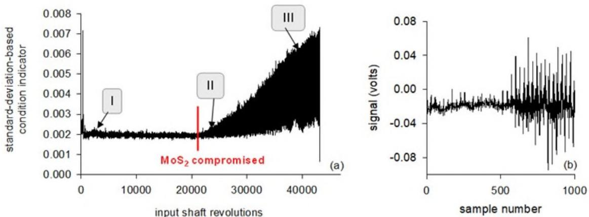
Figure 5. Typical trend and features of a condition indicator of MoS<sub>2</sub> film function. (a) Trend of condition indicator for the center distance (LVDT sensor), for test 1B. (b) Typical data record for calculation of standard-deviation-based condition indicator
