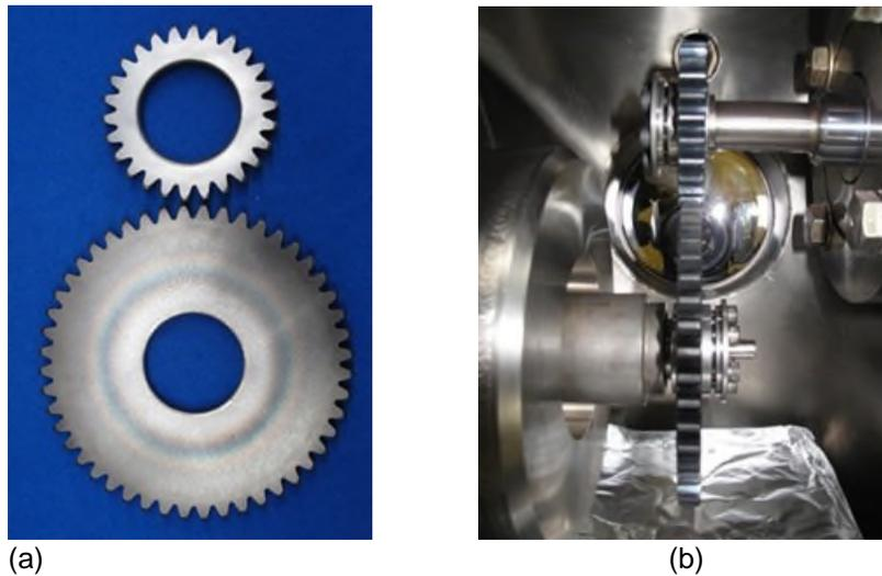
Figure 4. Test gears. (a) Just prior to testing. (b) Installed in rig just prior to closing of test chamber.
