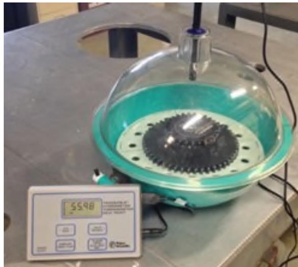
Figure 3. Humidity-exposure chamber for test gears.
