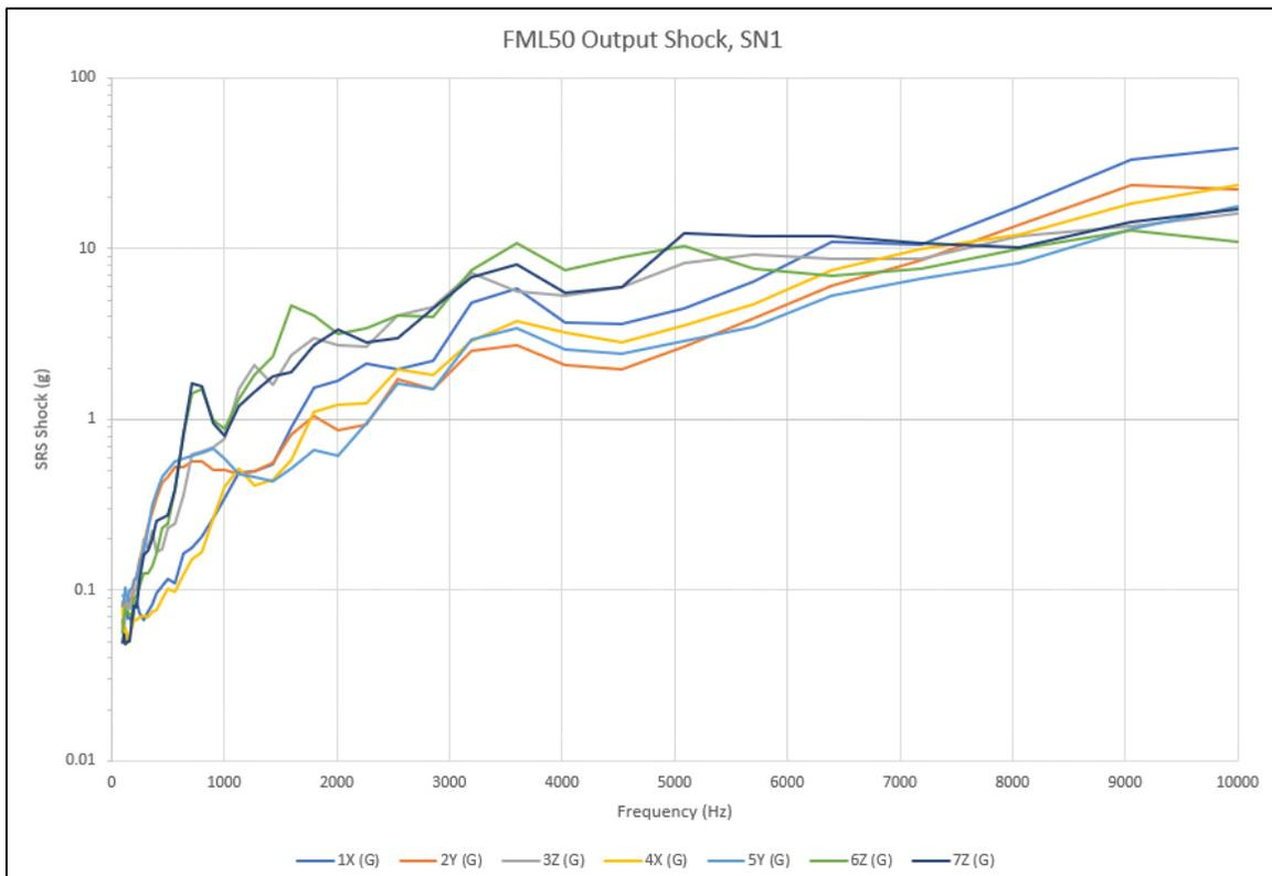
Figure 9. EBAD Thin Pack Output Shock Test Results.
