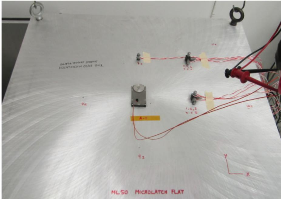
Figure 8. EBAD Thin Pack Output Shock Test Setup.
