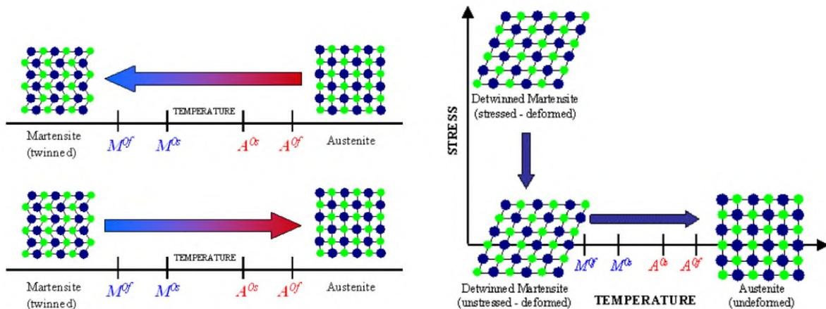
Figure 2. Shape Memory Alloy Phase Transformation [1]
