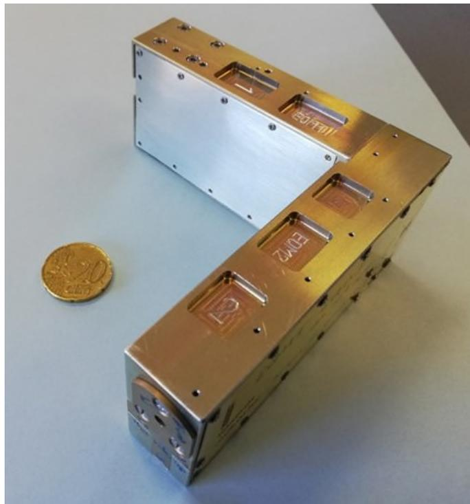
*Figure 8. Integrated two-axes GRASS instrument (without satellite interface and dummy BEE on the inside). Engraving in the mass reduction pockets allows clear identification of the instrument axes (1 and 2), as well as the instrument version (here: EQM). In the front, the bearings and encoder covers are visible. 20 cent euro coin for size-reference.*
