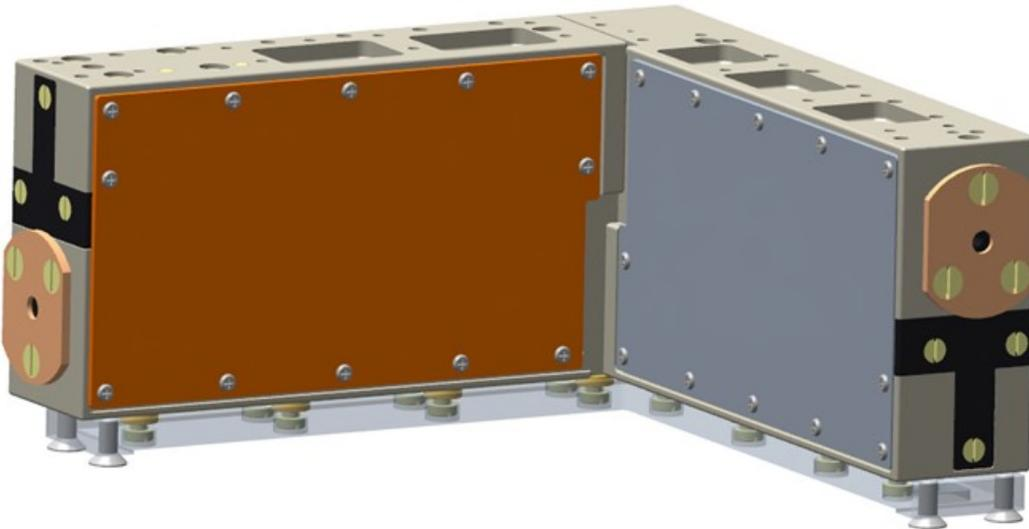
*Figure 3. Combination of two GRASS gravimeters to form an orthogonal setting. Clearly, the instruments appear identical but stacked upside-down to allow maximizing the length of the instrument. The two axes can be differentiated by the back-end electronics shown in orange and grey, respectively. On the bottom, the common mechanical interface plate is shown with the considered mounting screws for the Juventas CubeSat.*
