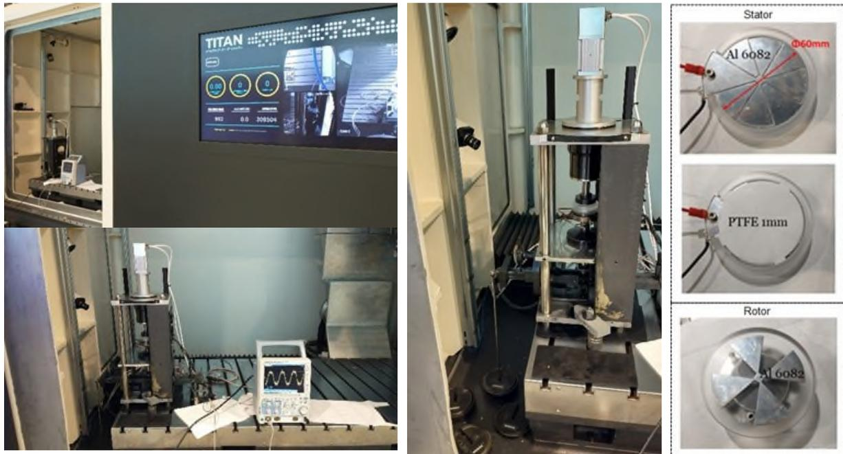
Figure 14. Test setup. Titan machine to reproduce Mars atmosphere, Falex rotatory tribometer, and manufactured trade-off breadboard to vary the power generation of the TEG.
