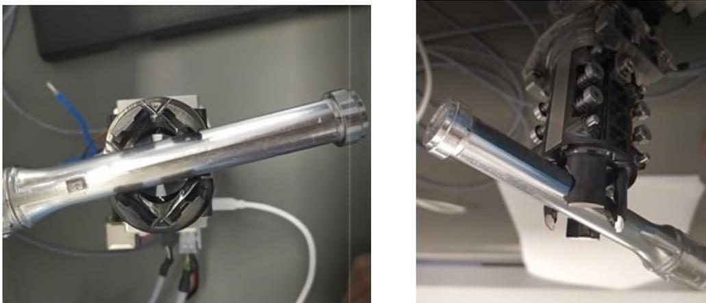
*Figure 16. Body-grip capture test (RSTA models courtesy NASA/JPL-Caltech).*
