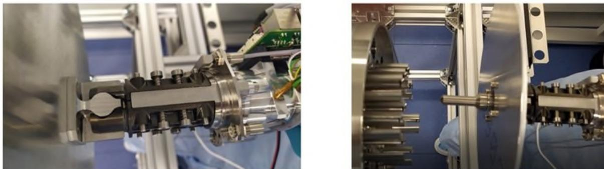
Figure 17. Grapple-Fixture Grasp of the OS-Lid Dummy.
