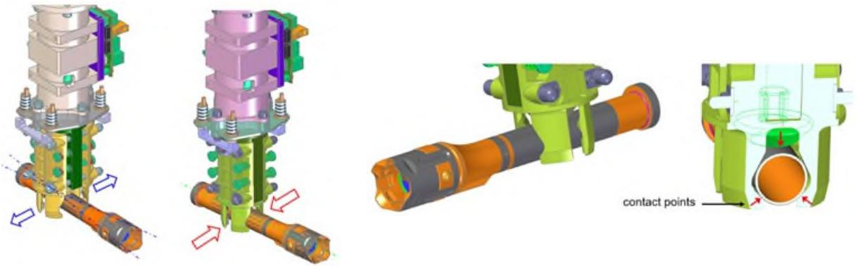
Figure 9. Body-Grip Grasp (RSTA model courtesy NASA/JPL-Caltech).
