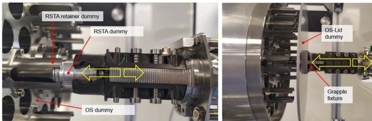
Figure 18. RSTA and OS-Lid Dummy Insertion and Extraction test.
