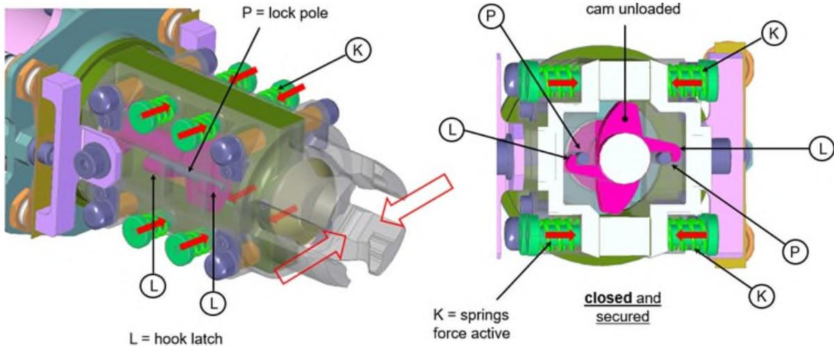
Figure 7. Closed Configuration.
