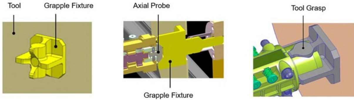
Figure 13. Grapple Fixture Design and Grasp.
