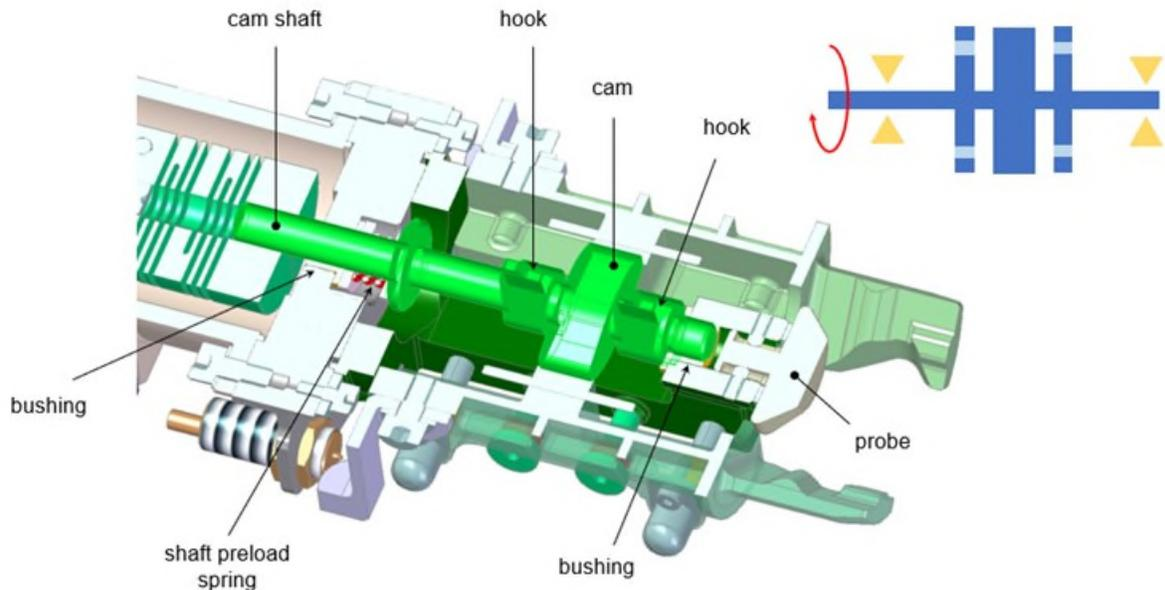
Figure 5. Gripper Cross Section and Cam Shaft Detail.
