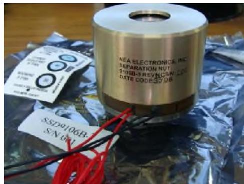
*Figure 4. NEA Release Device.*
