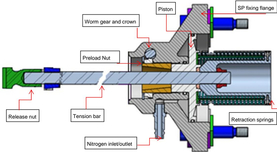
Figure 5. Detail of the pneumatic drive device.
