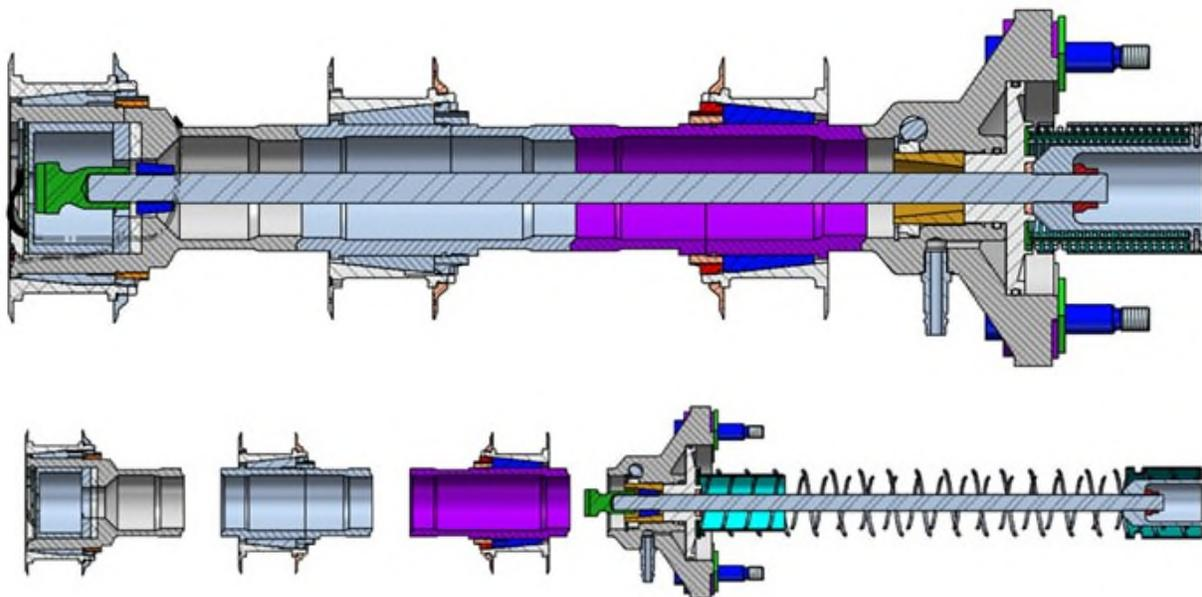
Figure 3. Restrain-Release Mechanism.
