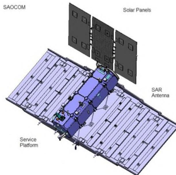
Figure 1. Flight configuration of the SAOCOM satellite.
