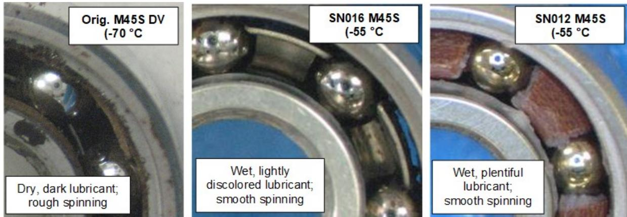
Figure 12 – Post-Life Condition of Front M45S Bearings
