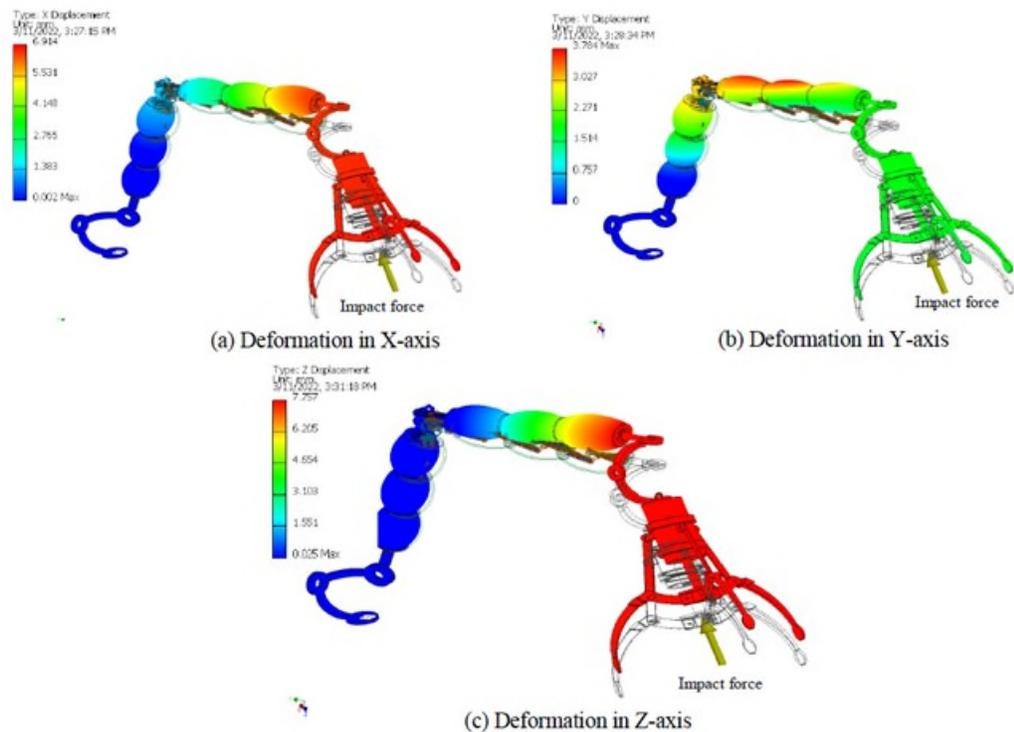
Figure 10. Deformation of a ERM-SOA due to impact force of 10 N at the end effector
