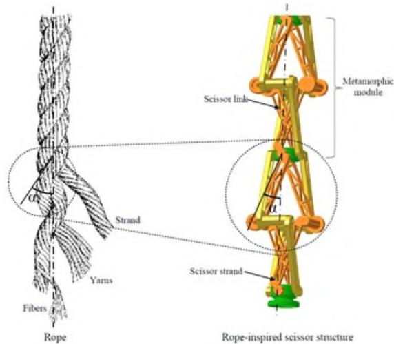
Figure 1. Rope-inspired scissor structure
