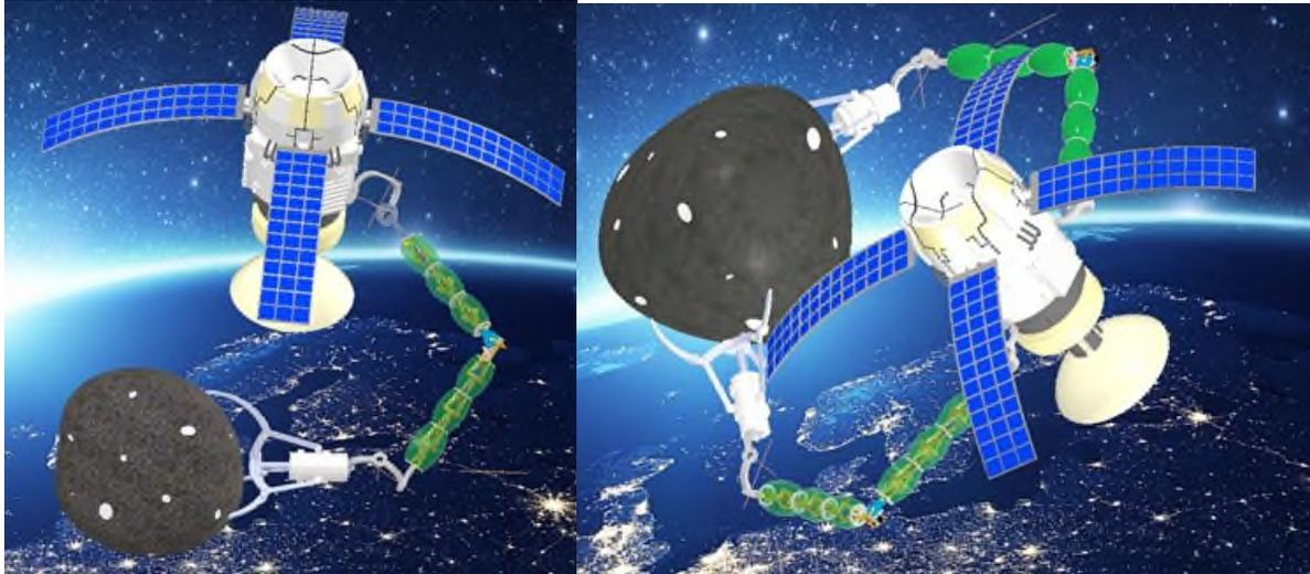
(a) Single space arm for capturing dead debris (b) Multiple space arms for capturing dead debris
