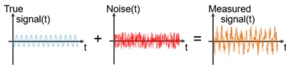
Figure 9: Schematic of a Measurement Signal Affected by Noise
