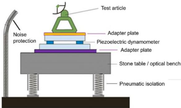
Figure 7: Typical Installation of Dynamometer for EFT Testing
