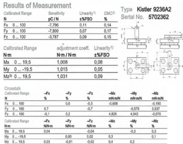
Figure 11: Example of a Calibration Certificate incl. Crosstalk and Linearity
