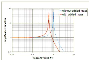
Figure 8: Natural Frequency of Spring Mass System
