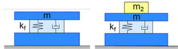
Figure 7: Spring Mass Model of PE Dynamometer
