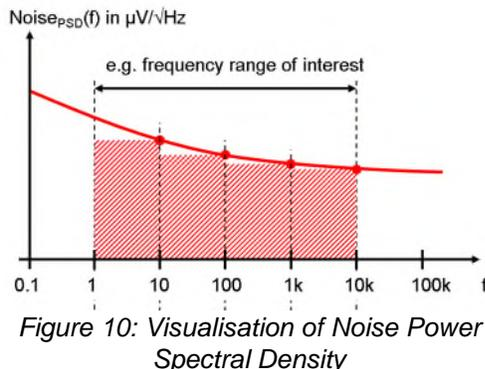
Figure 10: Visualisation of Noise Power Spectral Density
