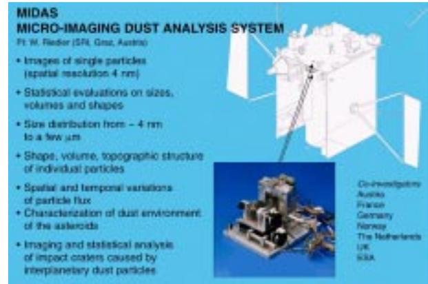
Figure 1 : Rosetta / Midas space mission (courtesy of ESA)
