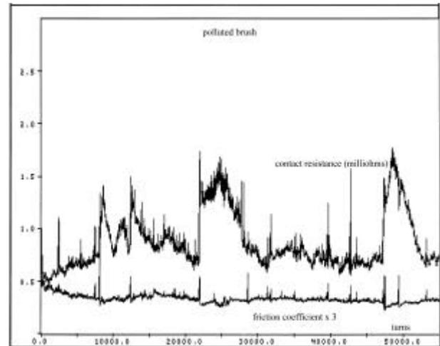
Figure 4.1.1 – Contact resistance and friction coefficient for the polluted brush, Vs number of turns
