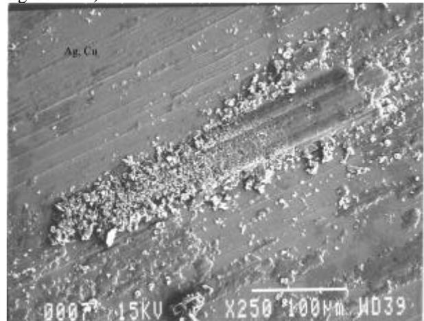
Figure 4.3.4 – SEM observation of the slip-ring under not polluted brush, after endurance test (SEI x 250)
