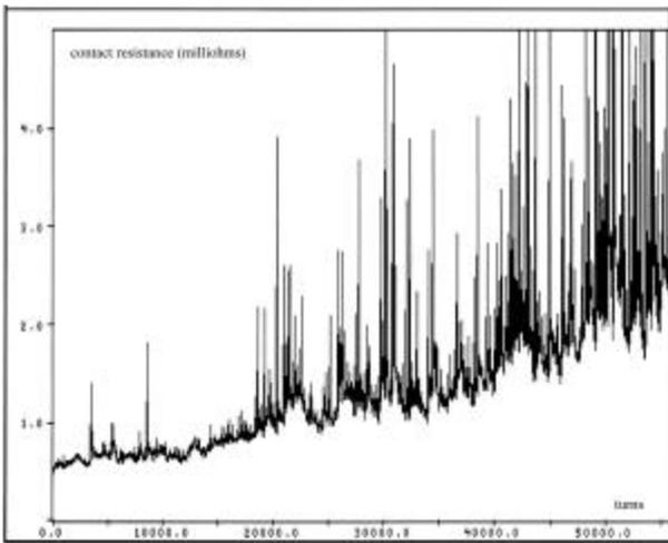
Figure 4.2.1 – Contact resistance of polluted brush at  $P = 10^{-6}$  mbar
