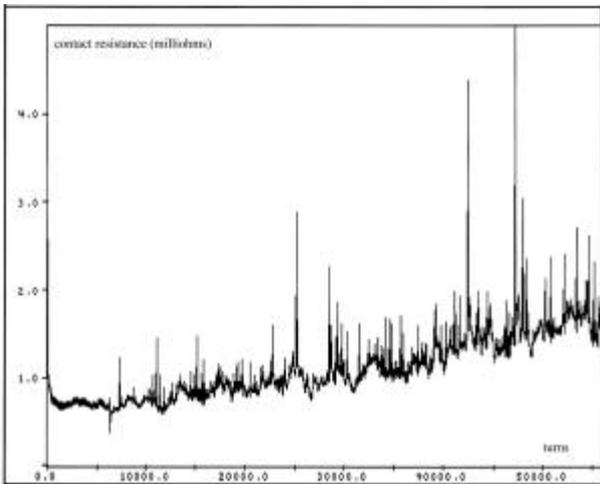
Figure 4.2.2 – Contact resistance of polluted brush at  $P = 10^{-5}$  mbar
