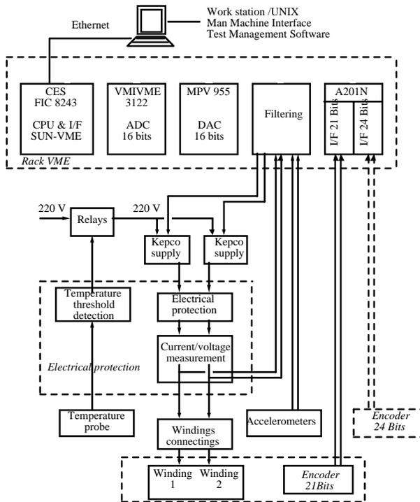
Figure 5 : A specific real time test bench allowed carrying out fine MCV’s characterisation
