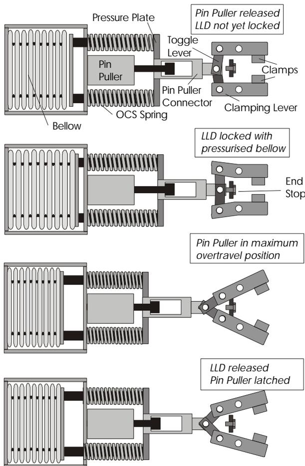
Figure 4: Schematic representation of the LLD function
