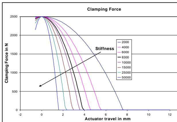
Figure 6: Clamping Force
