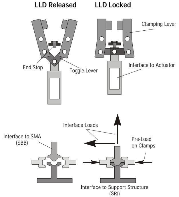
Figure 2: Principle design of LLD mechanism
