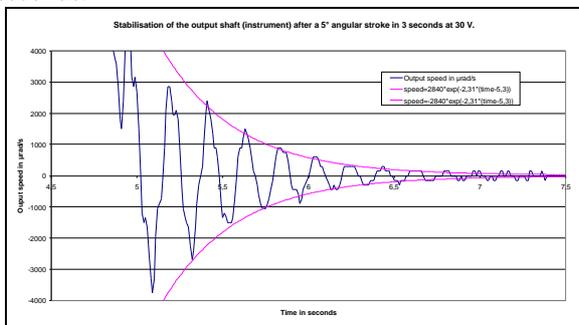
Figure 11: instrument stabilisation
