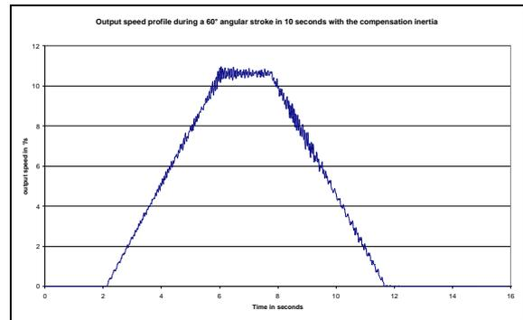
**Figure 9: output speed profile**
