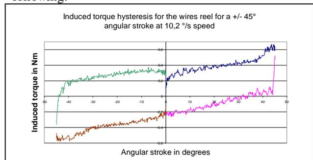
**Figure 3: Induced torque in the wires reel**
